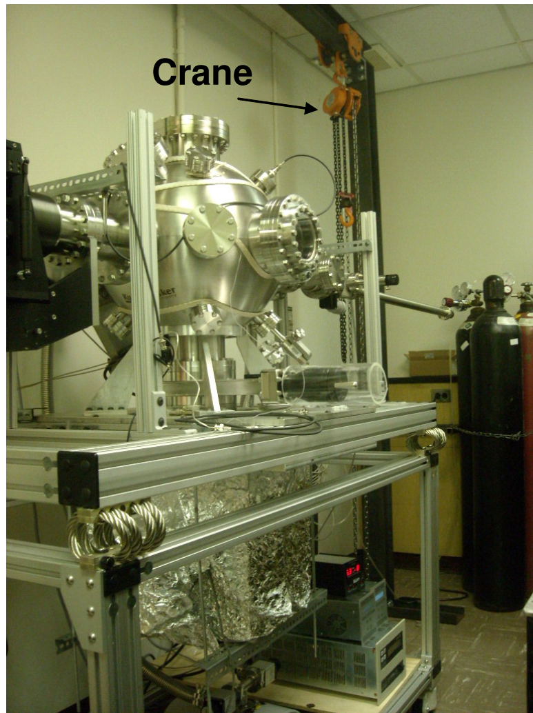
Figure A.7: Isometric view of the system. Electronic controllers, assembly crane and nitrogen tanks are visible.
