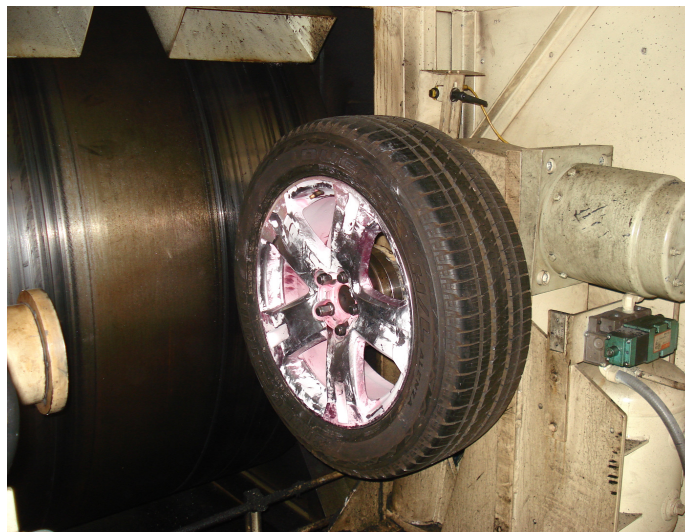
Figure 4-7. Radial fatigue test setup
