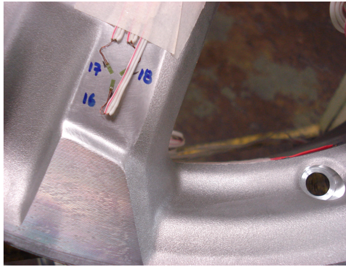
Figure 4-6. Strain gauges at location 6, spoke
