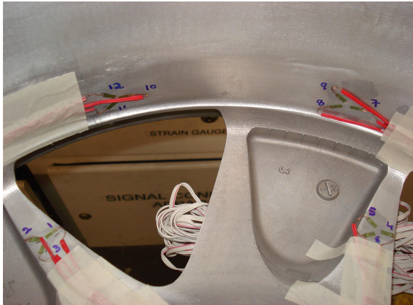
Figure 4-4. Strain gauges at locations 1 to 4
