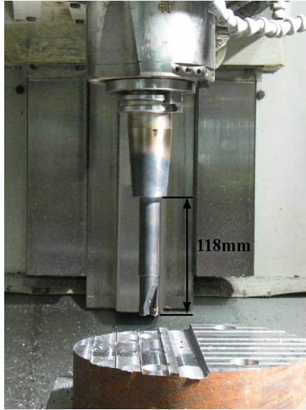
Figure 5-3: Setup for milling stability test
