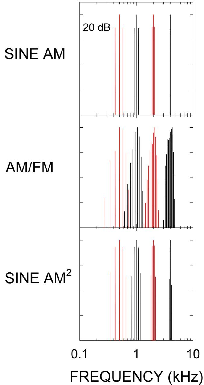
*Figure 1.1.* Acoustic spectra of stimuli used in this study (AM, AM/FM, and AM<sup>2</sup>) for carrier frequencies of 0.5, 1, 2, and 4 kHz. Y axis ticks represent 20 dB intervals.
