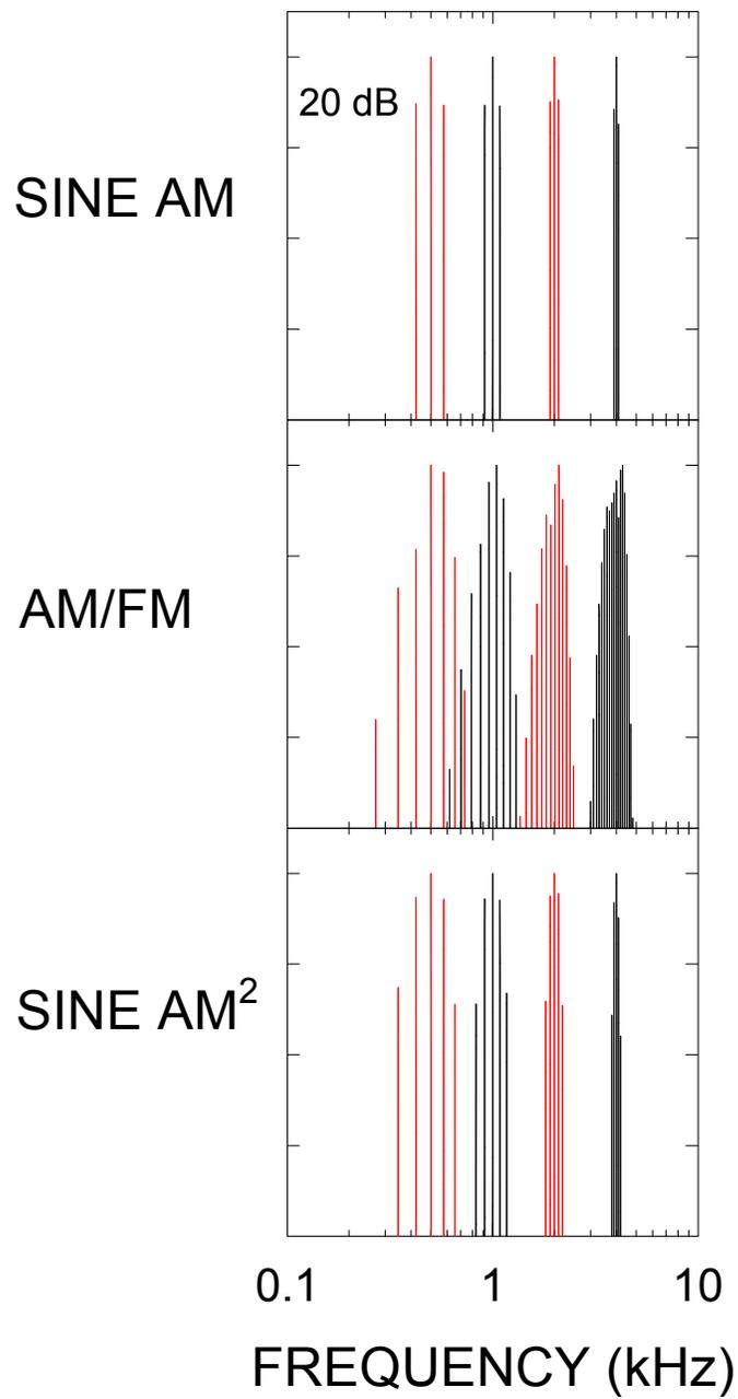
*Figure 2.1.* Acoustic spectra of stimuli used in this study (AM, AM/FM, and AM<sup>2</sup>) for carrier frequencies of 0.5, 1, 2, and 4 kHz. Y axis ticks represent 20 dB intervals.
