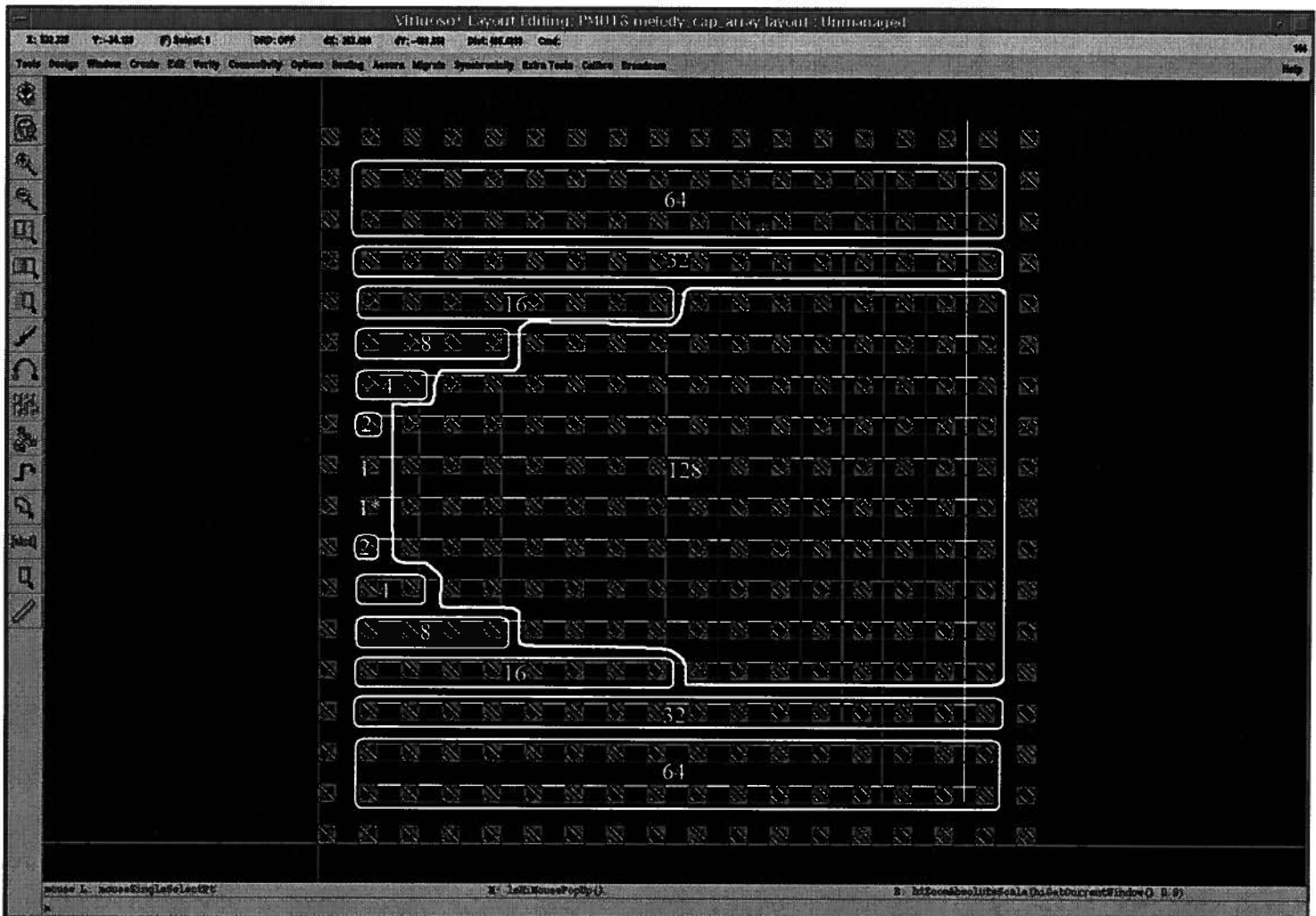
Figure 5-3. Capacitor array layout
