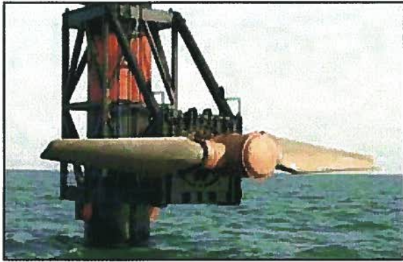
Figure 1-8: Horizontal axis tidal turbine (Courtesy of Marine Current Turbine Ltd.)
