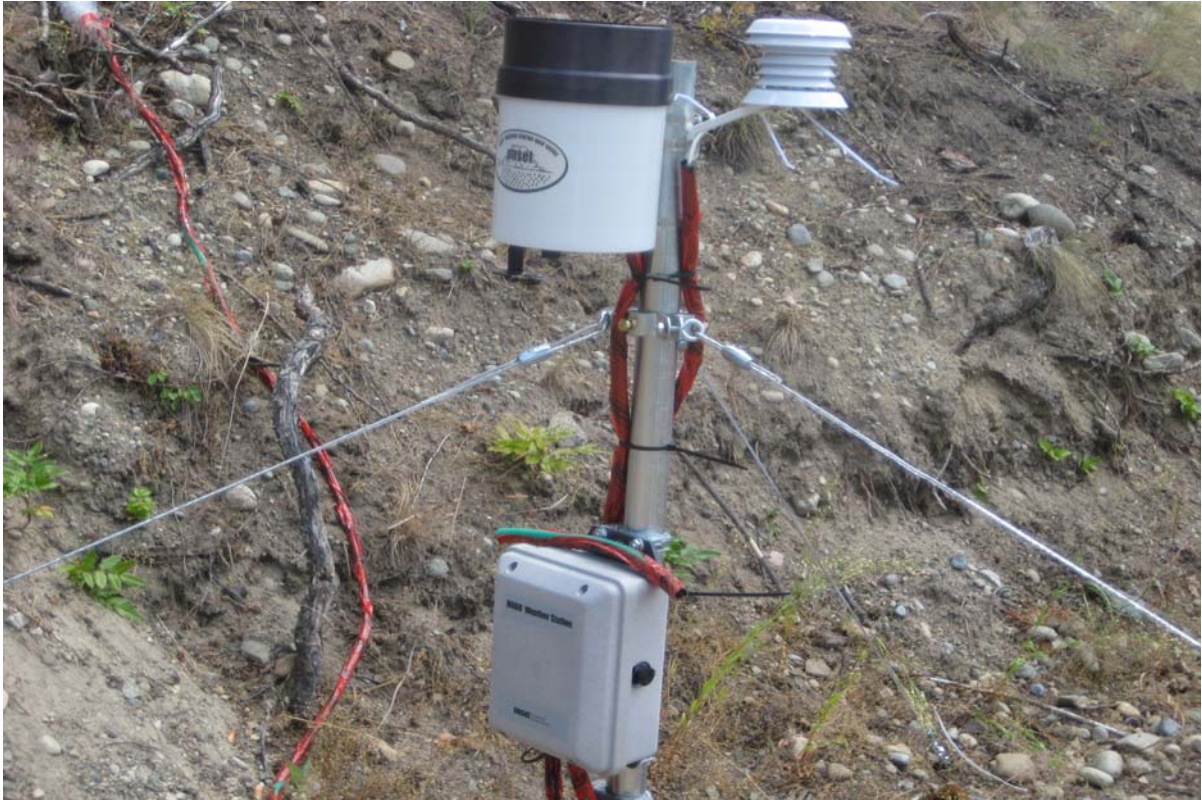
Figure 3.5 Weather station installed at the Wollemi Pine planting area to log information about local temperature, rainfall, relative humidity, and soil moisture.
