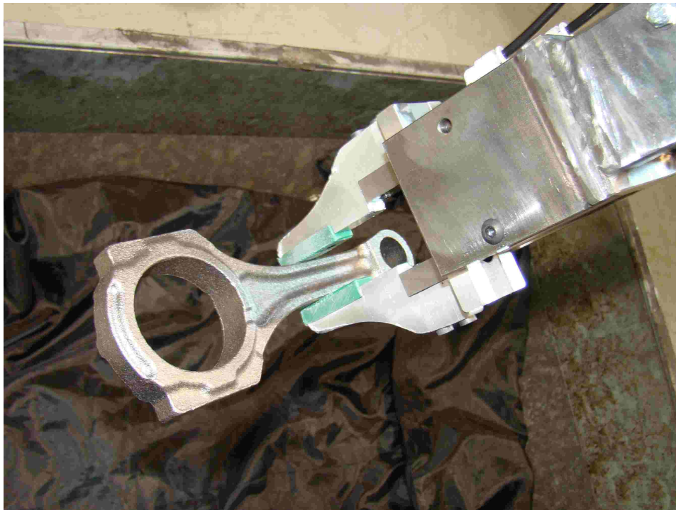
Figure 1.1: Standard industrial two-fingered (antipodal) gripper using a nominal grasp to grip a connecting rod, or con-rod [17].
