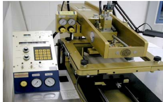
Figure 2-5 Screen printing (left- a schematic of the printing process, right- the screen printer used in this study, MC 212 Screen Printer).
