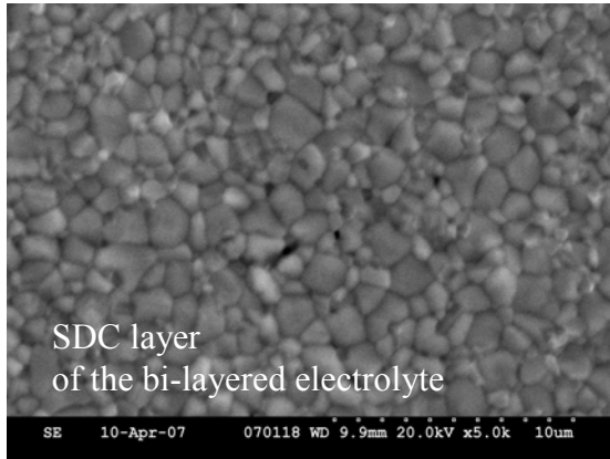
Figure 8-1 SEM image of the bi-layered SDC/SSZ electrolyte surface
