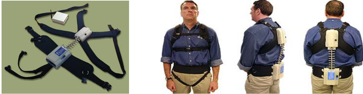
Figure 1.2 LMM components (left), front, lateral and back views of LMM worn on by an individual (right). Original images taken from NexGen Ergonomics Inc (NexGen Ergonomics Inc., 2007).
