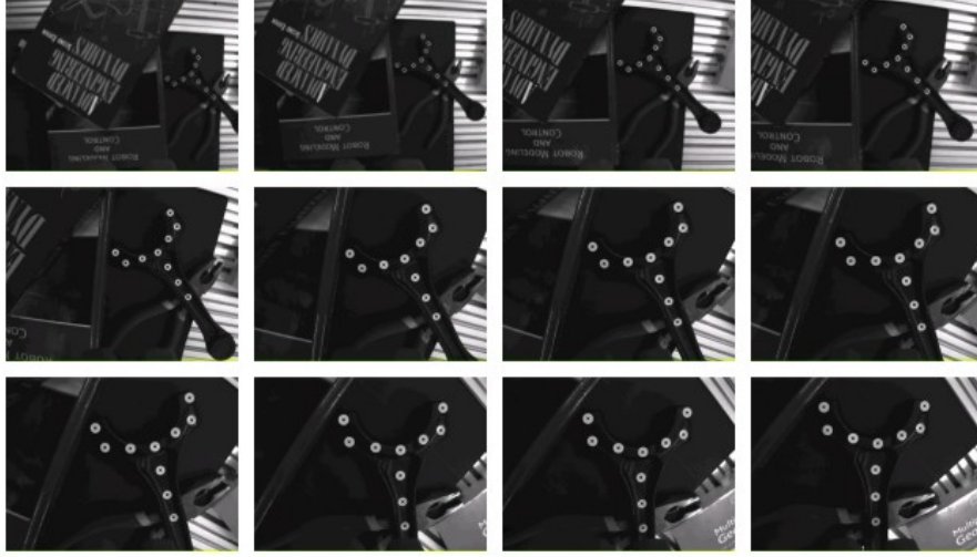
Figure 6.19: Sequence of camera motions generated by MPC visual servoing to complete a difficult positioning task. The resulting image feature trajectories satisfy the camera field-of-view constraints.
