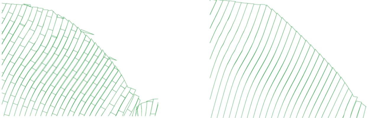
**Figure 4.29:** Self-stabilizing of rock blocks and potential catastrophic rock mass failure. (Magnified deformation - 10 times, Slope height – 800 meters)
