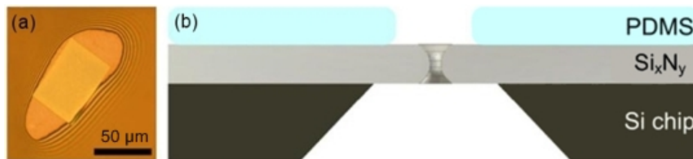
Figure 5.5: (a) Optical top view image of a PDMS coated nanopore chip showing the PDMS close to the freestanding membrane window (b) Cross-section of PDMS painted nanopore chip (not to scale)
