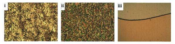
**Figure 3.44**: POM images of **34c** taken at a magnification of 10× i) 25 °C Cr ii) 125 °C N iii)140 °C I
