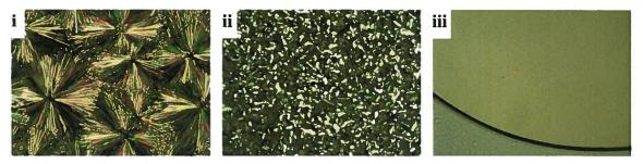
**Figure 3.40**: POM images of **23f** taken at a magnification of 20× i) 25 °C Cr ii) 62 °C N iii) 70 °C I
