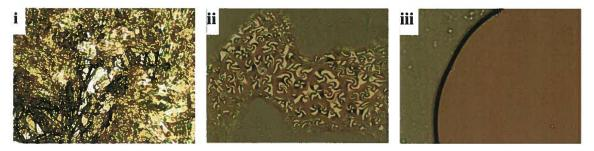
Figure 3.45: POM images of 34d taken at a magnification of 10× i) 25 °C Cr ii) 122 °C N iii) 140 °C I
