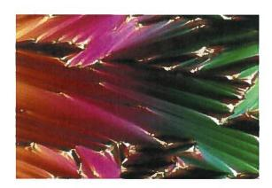
**Figure 1.4**: Representative texture of a smectic A liquid crystal (courtesy of M. Neubert; http://www.lci.kent.edu/fans.html).
