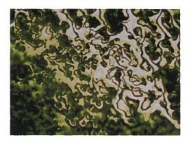
Figure 1.11: POM image of a nematic liquid crystal displaying birefringence.
