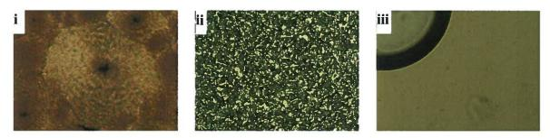
**Figure 3.41**: POM images of **23g** taken at a magnification of 20× i) 20 °C Cr ii) 25 °C N iii) 100 °C I
