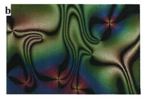
**Figure 1.1:** a) Schematic of a nematic liquid crystal, b) Representative texture of a nematic liquid crystal (courtesy of O. Lavrentovich; http://www.lci.kent.edu/defect.html).
