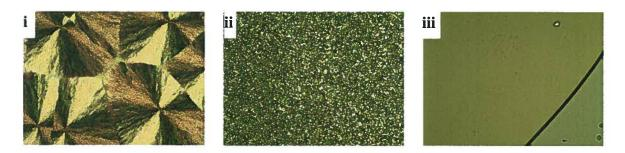
**Figure 3.39**: POM images of **23e** taken at a magnification of 20× i) 25 °C Cr ii) 55 °C N iii) 70 °C I
