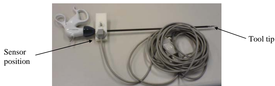
Figure 3.3: Tool tip and sensor locations. The tool tip motion is reported with respect to an instantaneous inertial reference frame is located at the sensor position
