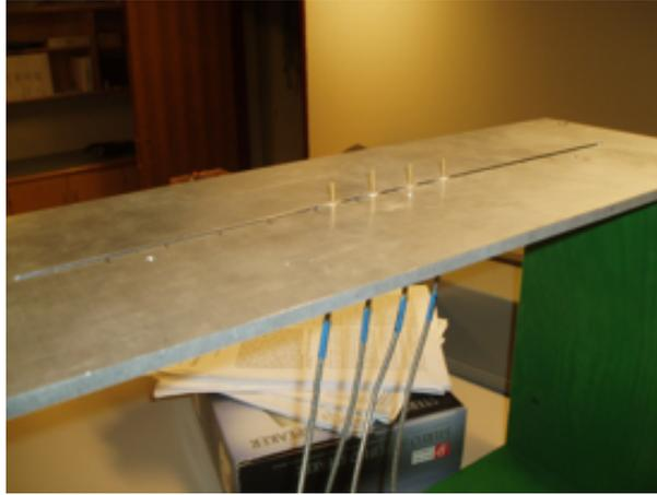
Figure 3.5: Photo of the four-antenna linear monopole array used for transmission and reception.
