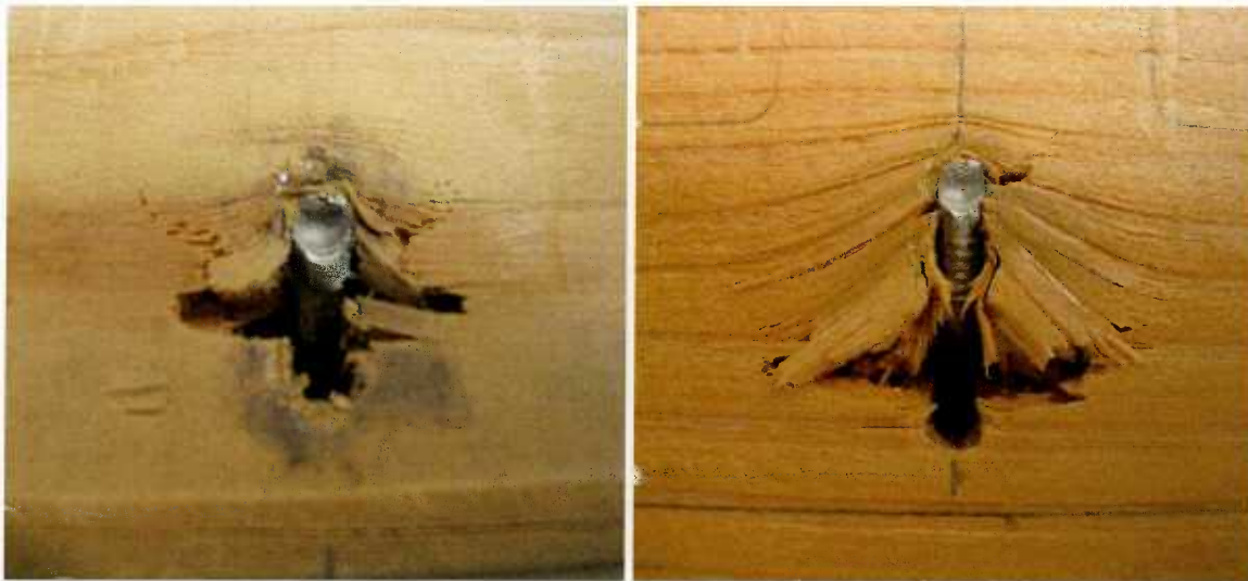
Figure 6.9 Localized wood crushing failure in the perpendicular to grain direction: nail on the tangential surface-PET (left), and nail on the radial surface-PER (right).
