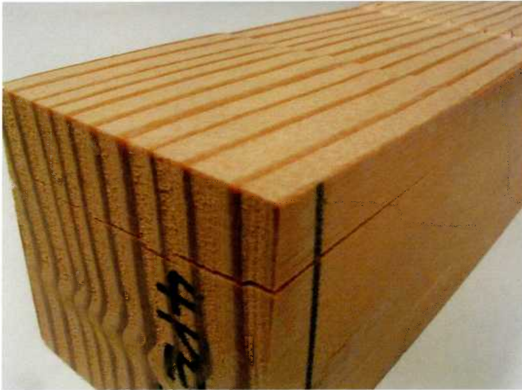
Figure 4.19 End split failure of the 2×2×6 perpendicular to grain compression specimen.
