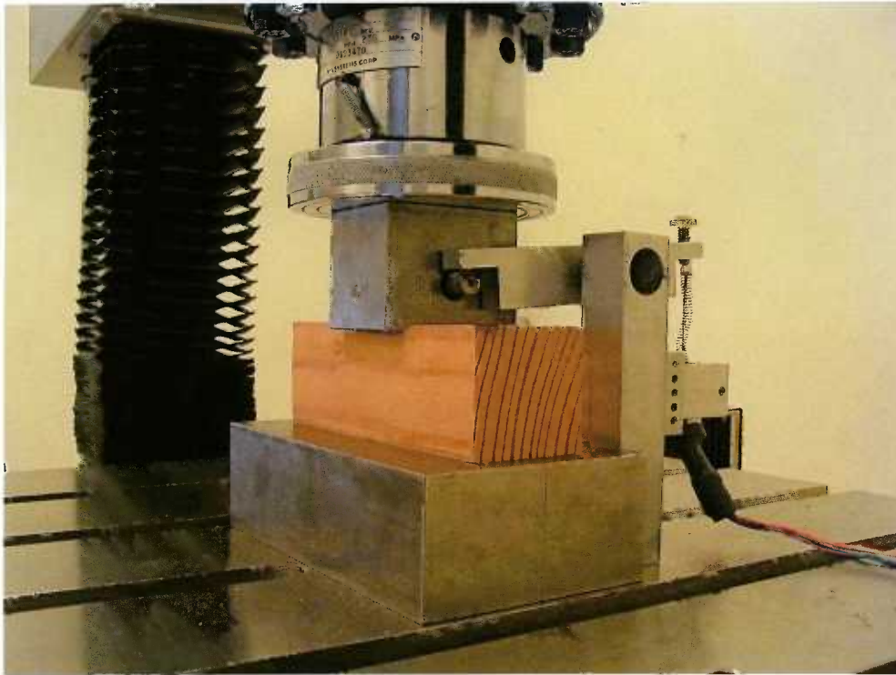
Figure 4.3 The conventional ASTM D 143 perpendicular to grain compression test.
