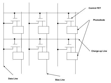
Figure 1-2: An array of photodiodes used for the flat panel imager is shown. Each photodiode collects visible photons generated by the high energy x-rays. The data are read out through the data line and the timing is controlled by the control FET. The bias line is used to control the bias to the photodiode and the charge-up line is used to control the opening and closing of the control FET.
