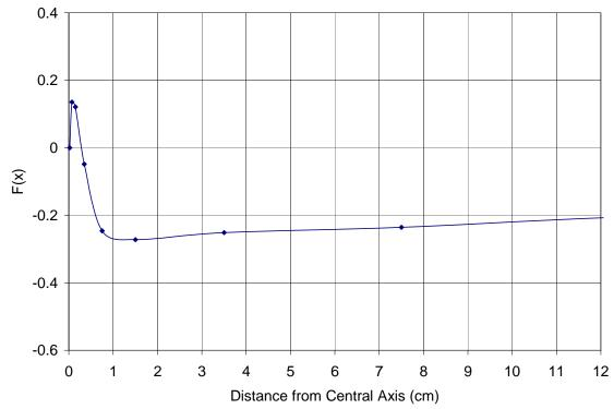
Figure 3-6: The relative scatter factor, F(x), of the two 6MV scatter kernels. The 2100EX and Mohan are the  $k_{s,base}$  and  $k_s$  respectively.
