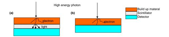
Figure 1-1: Two types of radiation detectors are shown here. (a) Indirect detector converts incident radiation into secondary electrons which are converted into visible light for detection; (b) Direct detector converts radiation directly into secondary electron for detection.
