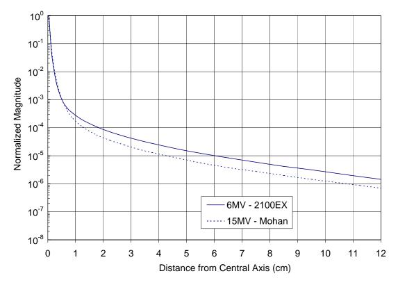
Figure 3-7 : Normalized profiles of flat panel EPID scatter kernels for 6MV (solid) and 15MV (dotted) beams.
