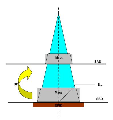
Figure II-1 flat panel imager, EPID, measures a profile at Source to Detector Distance (SDD),  $M_{SDD}$ , which is back-projected to SAD to become  $M_{SAD}$ .
