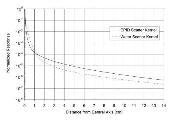
Figure 3-9: Scatter kernel profile of the flat panel EPID (solid) with no build-up material and water phantoms (dotted) at a depth of 1.5 cm with 6MV beam
