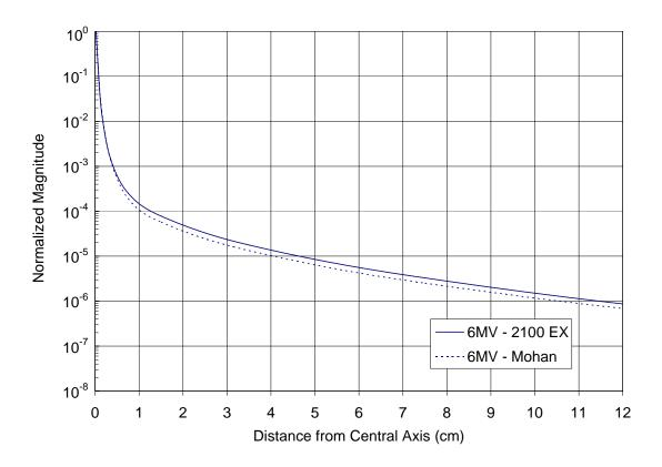
Figure 3-5: EPID scatter kernel profiles of 6MV beam generated from Clinac 2100 EX (solid) and Mohan (dotted) spectra are shown.
