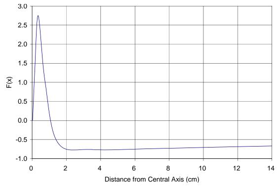
Figure 3-10: Relative scatter factor of water kernel relative to the flat panel EPID kernel at 6MV. The flat panel EPID kernel and water kernel are the  $k_{s,base}$  and  $k_s$  respectively.
