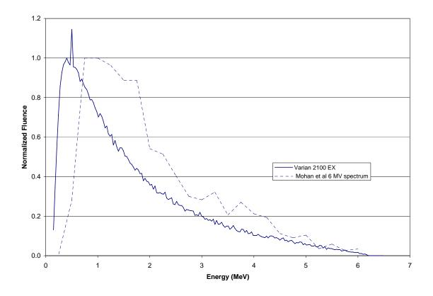
Figure 3-3: The energy spectrum of the 6MV photon beam of Clinac 2100 EX calculated with BEAMnrc (solid) and the 6MV Mohan's spectrum is included for comparison (dotted).
