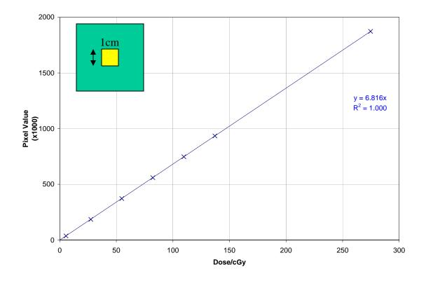
Figure 3-2: The response of the flat panel EPID as a function of dose for a field size of  $10x10 \text{ cm}^2$
