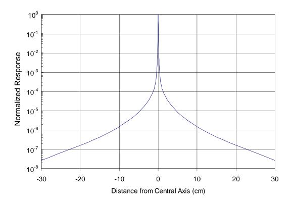
Figure 3-4: A semilogarithmic plot of the spatial response of the scatter kernel of the flat panel EPID from a 6MV non-diverging pencil beam calculated with DOSRZnrc
