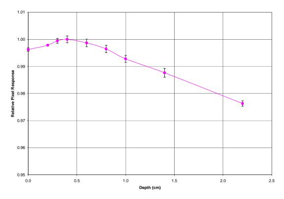
Figure 3-1: Depth response of the imager taken from 0 cm to 2.3 cm of water. The measurements are normalized to 0.4 cm. The error bars represent one standard deviation of the measurements.
