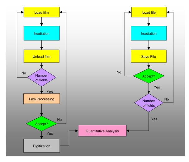
Figure 1-4: Flow charts of film based verification and EPID-based verification. It shows that the number of steps involved in each process.
