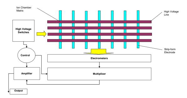
Figure I-1 This shows a schematic of a SLIC EPID. High voltage switches turn on the high voltage lines one at a time to turn on the horizontal array of ion chambers. The readings are read out via the electrometers which are multiplexed and sent to output via an amplifier.
