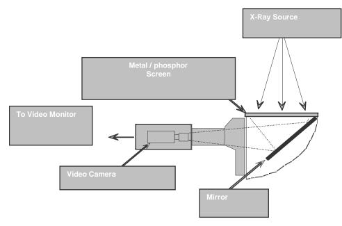
Figure I-2: Video-based EPID consists of a video camera store connected to a video monitor outside the treatment room. A metal/phosphor screen is used for converting x-ray to visible light which is directed to the camera via a mirror.
