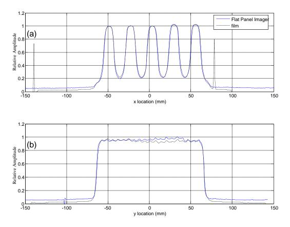
Figure 3-14: (a) Calibrated flat panel EPID and film profiles along the x-direction; (b) calibrated flat panel EPID and film profiles along the y-direction.
