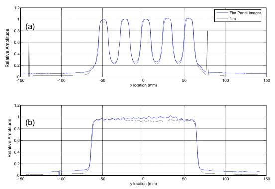
Figure 3-13: (a) Flat panel EPID and film profiles along the x-direction; (b) flat panel EPID and film profiles along the y-direction.
