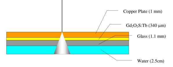
Figure 2-2: The flat panel EPID phantom model used in DOSXYZnrc and DOSRZnrc
