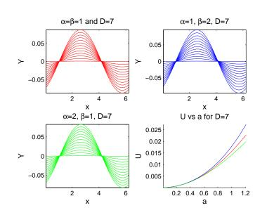
Figure 3.5: Solution for viscoelastic elastic lubrication problem for various fluid types with D=7. Red: Newtonian. Blue: Shearing Thinning. Green: Shear Thickening.
