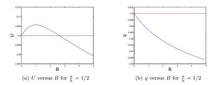
Figure 2.9: Swimming speed and mass flux for varying Bingham number. The corresponding Newtonian values are shown in red.
