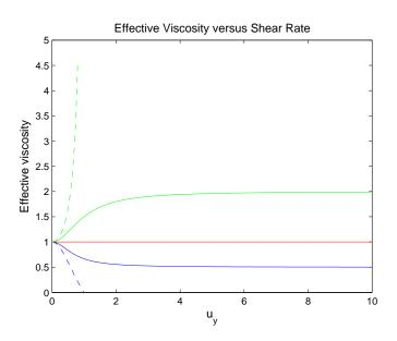
Figure 2.2: Effective Viscosities. Red: Newtonian, Solid Blue: Shear Thinning, Dashed Blue: Unrealistic Shear Thinning, Solid Green: Shear Thickening, Dashed Green: Unrealistic Shear Thickening
