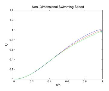
Figure 2.3: Non-Dimensional Swimming Speeds. Red: Newtonian. Blue: Shearing Thinning. Green: Shear Thickening.
