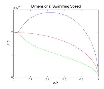
Figure 2.4: Dimensional Swimming Speeds. Red: Newtonian. Blue: Shearing Thinning. Green: Shear Thickening.
