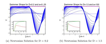
Figure 3.2: Newtonian Solution of Elastic Lubrication Problem. In the bottom left hand corner of each figure we see the swimming speed (red) and the mass flux (green) versus the forcing amplitude. The magenta horizontal lines are the calculated plateau values for each case.
