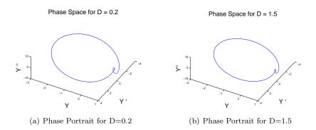
Figure 3.3: Phase portraits for Newtonian Solution of Elastic Lubrication Problem with large amplitude forcing.
