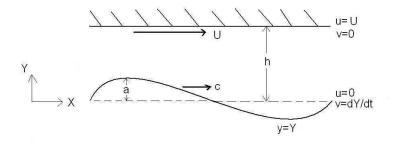
Figure 1.2: Geometry of Problem in Moving Frame of Reference
