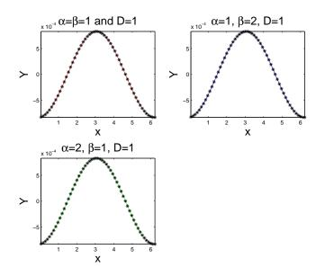
Figure 3.7: Comparison between analytical and numerical results for low amplitude swimming problem. Numerical results are solid lines, analytical results are shown by \*. Red: Newtonian. Blue: Shearing Thinning. Green: Shear Thickening.
