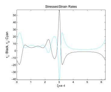
Figure 3.9: Strain rates on the swimmer (cyan) and on the wall (black) for a=100 and D=1.5. Note that the largest strain rates occur in the region where the plateau ends and the spike begins.
