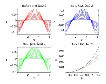
Figure 3.4: Solution for viscoelastic elastic lubrication problem for various fluid types with D=0.2. Red: Newtonian. Blue: Shearing Thinning. Green: Shear Thickening.
