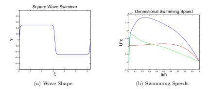
Figure 2.10: Example of alternate wave shape and resulting swimming speeds. Red: Newtonian. Blue: Shearing Thinning. Green: Shear Thickening.
