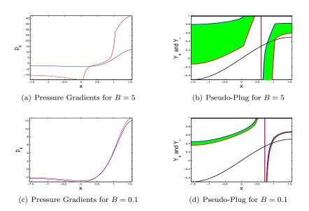
Figure 2.8: Pressure Gradients and Yield Surfaces for large and small B,  $\frac{a}{h} = 1/2$ . In the left figures, the Newtonian pressure gradient is blue, the Bingham red. In the right figures,  $Y_+$  is blue,  $Y_-$  is red, and the shaded green represents the pseudo-plugs. The surface of the swimmer is represented by the black curve and the pink vertical line shows where the pressure gradient changes sign.
