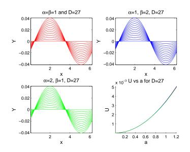
Figure 3.6: Solution for viscoelastic elastic lubrication problem for various fluid types with D=27. Red: Newtonian. Blue: Shearing Thinning. Green: Shear Thickening.
