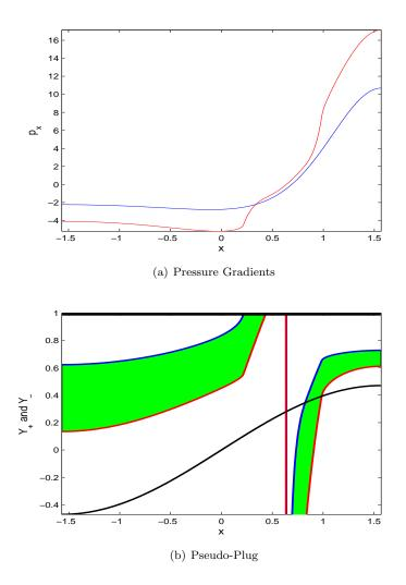
Figure 2.6: Pressure Gradients and Yield Surfaces for B = 1 and  $\frac{a}{h} = 1/2$ . The Newtonian pressure gradient is blue, the Bingham red. In the lower figure,  $Y_+$  is blue,  $Y_-$  is red, and the shaded green represents the pseudo-plug. The surface of the swimmer is represented by the black curve and the pink vertical line shows where the pressure gradient changes sign.
