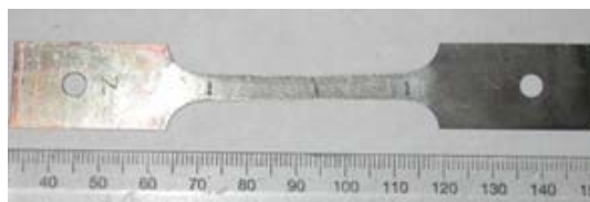
Figure 70: 316 sample 2 tested as received
