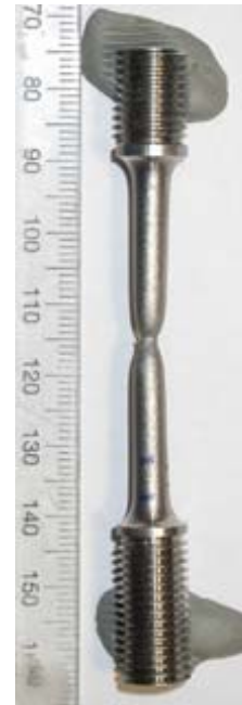
Figure 35: 316L tested in 25 MPa H 2 at -40°C
