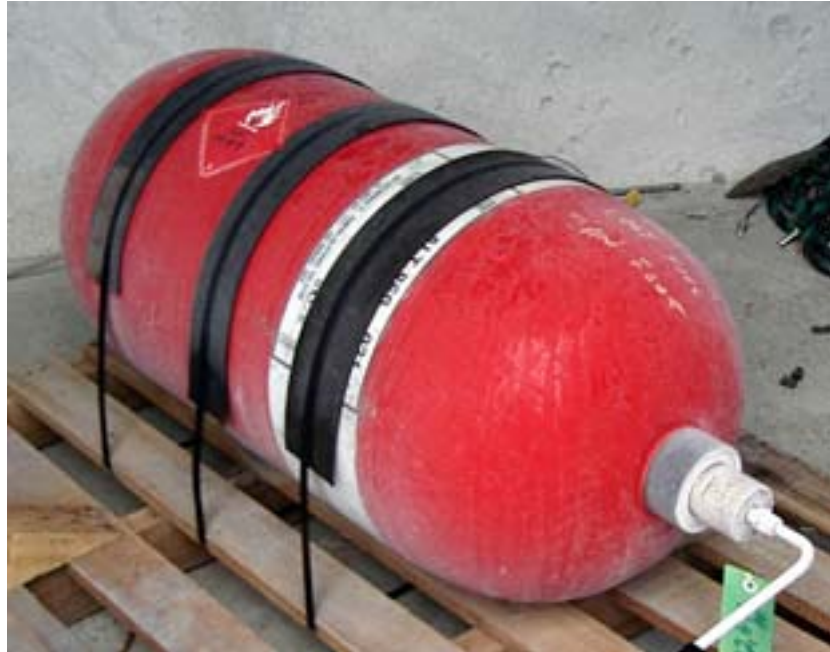
Figure 1: Carbon fibre fully wrapped tank with SS 316 liner
