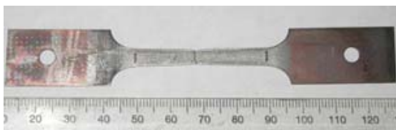
Figure 69: 316 sample 1 tested as received
