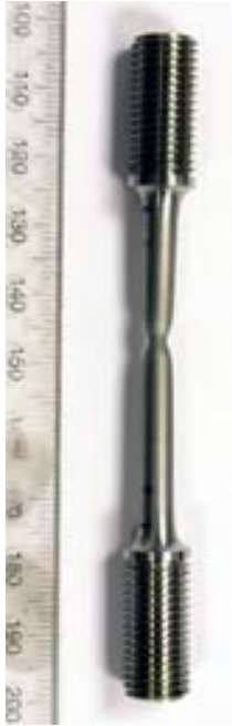
Figure 32: 316L tested in 25 MPa He at 20°C
