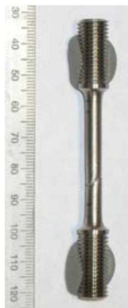
Figure 31: 316 tested in 25 MPa H 2 at -40°C
