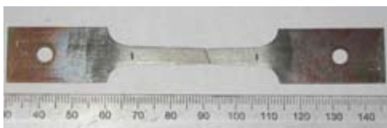
Figure 75: 316L sample L1 tested as received
