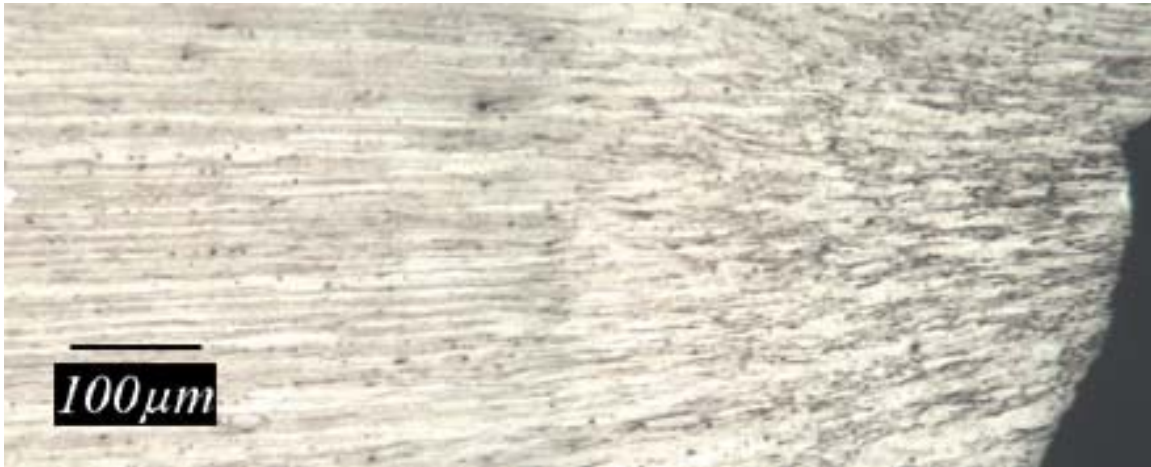
Figure 48: Example of martensite distribution in hydrogen environment tensile sample
