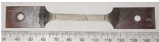
Figure 77: 316L sample L3 charged in 100°C air
