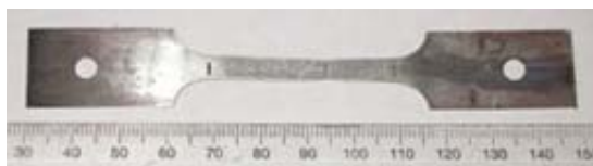
Figure 74: 316 sample 6 charged in 100°C H 2
