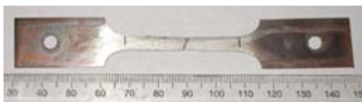
Figure 71: 316 sample 3 charged in 100°C air
