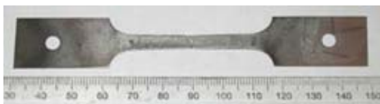
Figure 73: 316 sample 5 charged in 100°C H 2
