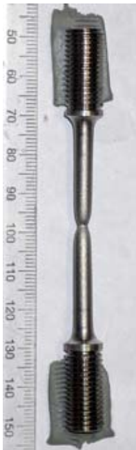
Figure 34: 316L tested in 25 MPa He at -40°C
