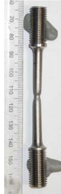
Figure 33: 316L tested in 25 MPa H 2 at 20°C
