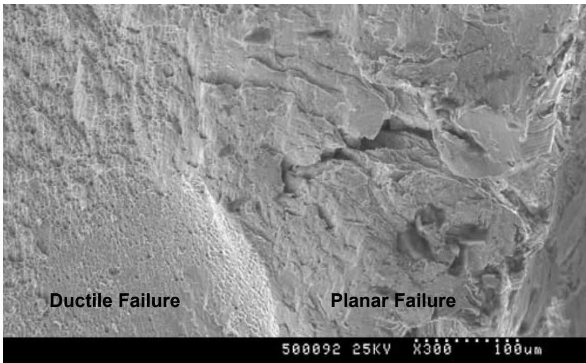
Figure 67: 316L tested in 25 MPa H 2 at -40°C showing brittle-to-ductile transition (300x)
