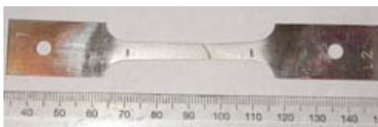
Figure 76: 316L sample L2 tested as received
