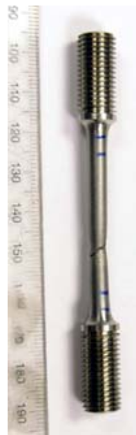
Figure 29: 316 tested in 25 MPa H 2 at 20°C
