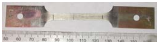
Figure 78: 316L sample L4 charged in 100°C air
