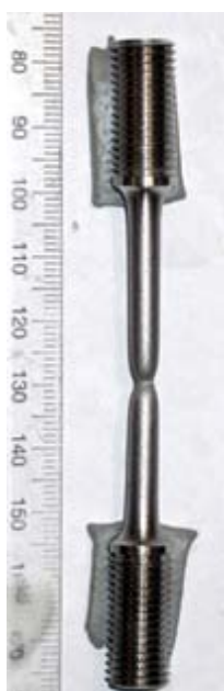
Figure 30: 316 tested in 25 MPa He at -40°C
