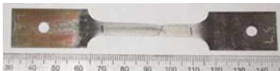
Figure 80: 316L sample L6 charged in 100°C H 2
