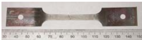
Figure 79: 316L sample L5 charged in 100°C H 2
