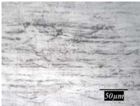
Figure 49: 316 tested in 25 MPa He at 20°C showing very little martensite (200x)
