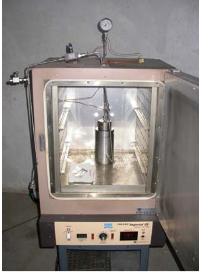
Figure 18: High-temperature hydrogen charge apparatus
