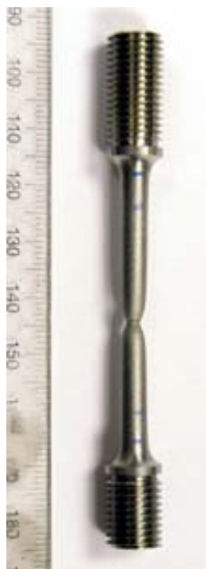
Figure 28: 316 tested in 25 MPa He at 20°C
