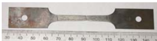
Figure 72: 316 sample 4 charged in 100°C air
