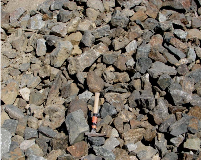
Figure 5 – Low grade stockpile at Pipe. Note the relatively consistent particle size distribution of the rocks in the sample.
