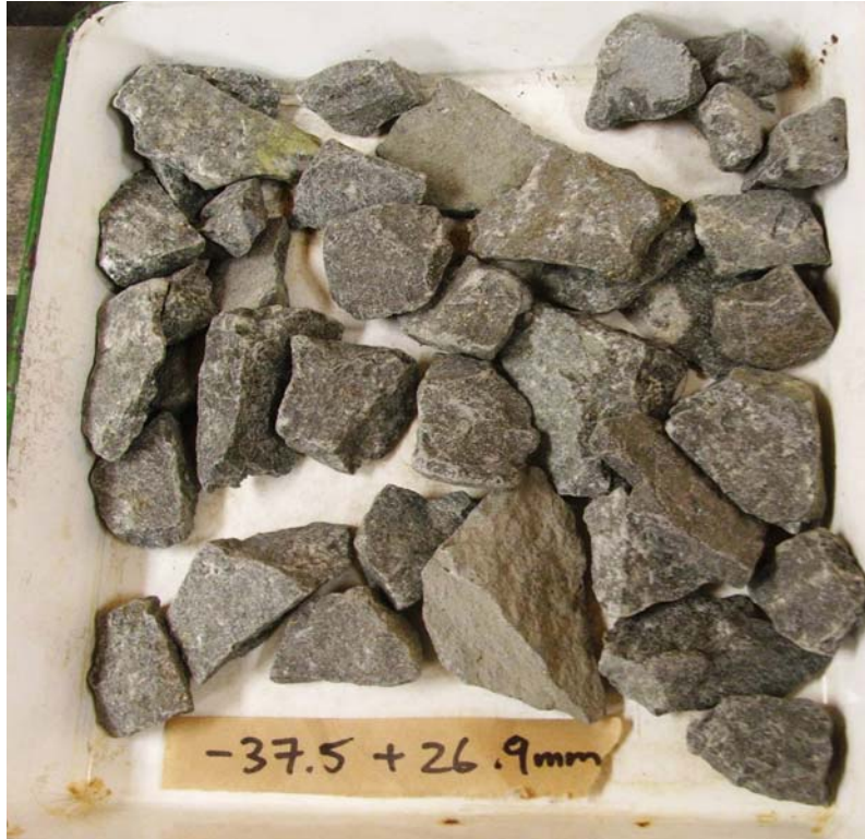
Figure 6.14 – Typical Dense Medium Separation Reject fraction (Fraser Ni)
