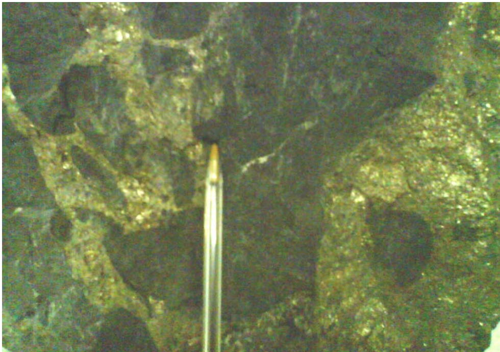
Figure 3 – Photograph of intraparental brecciated sulphide sample from Pipe. Note massive / net textured sulphides with incorporated schist inclusions
