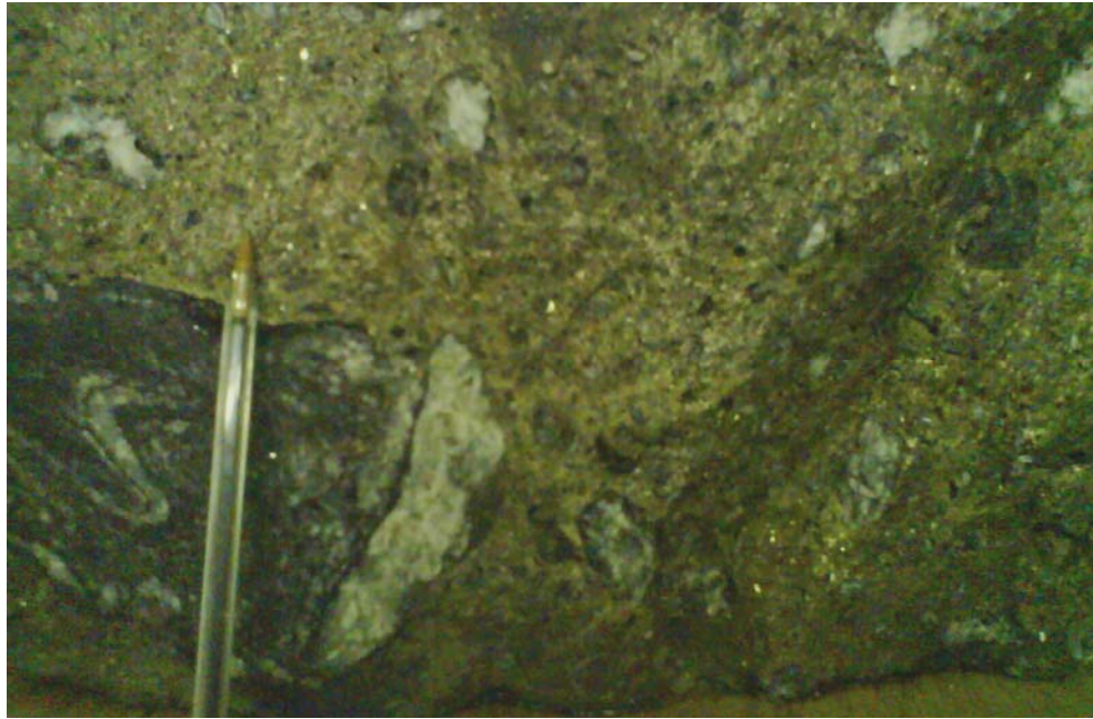
Figure 6.24 –Extraparental massive sulphide sample at Pipe. Note highly foliated nature of breccia inclusions that mimic the overall structural geology of the TNB
