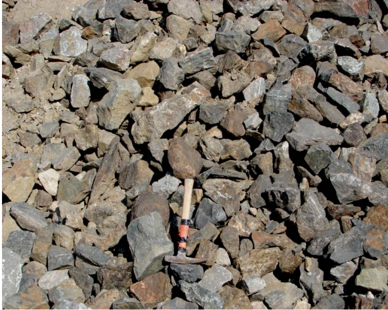
Figure 6.26 – Low grade stockpile at Pipe. Note the relatively consistent particle size distribution of the rocks in the sample.
