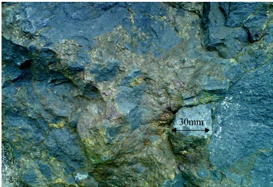
Figure 6.12– Sudbury breccia /matrix type ore texture
