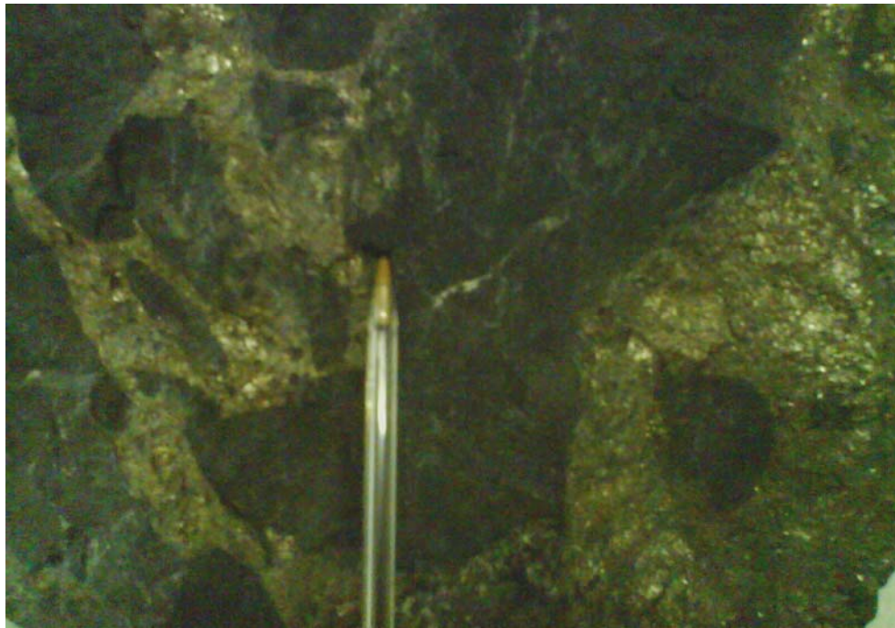
Figure 6.25 – Photograph of intraparental brecciated sulphide sample from Pipe. Note massive / net textured sulphides with incorporated schist inclusions
