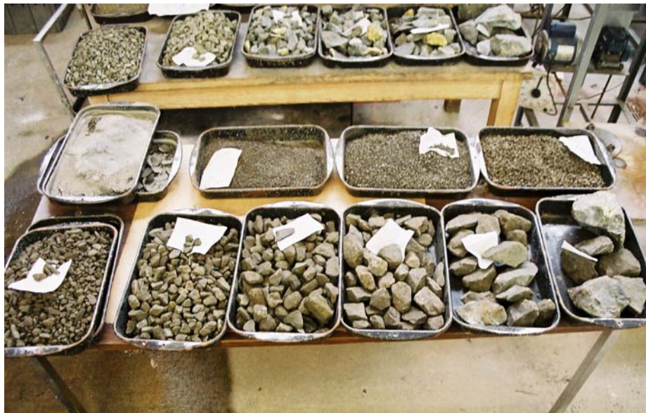
Figure 4.3 – Screened Sample Fractions for Size Assay
