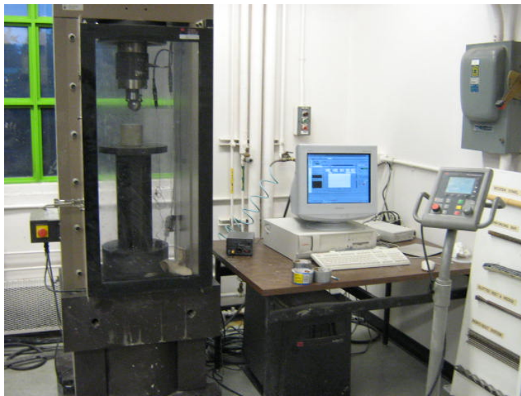
Figure 4.17 – MTS 815 UCS Testing Machine
