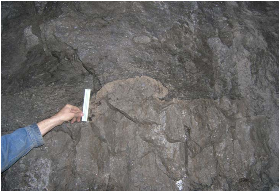
Figure 6.2 – Close up of breccia type ore in-situ showing sharp contact with the dolomites
