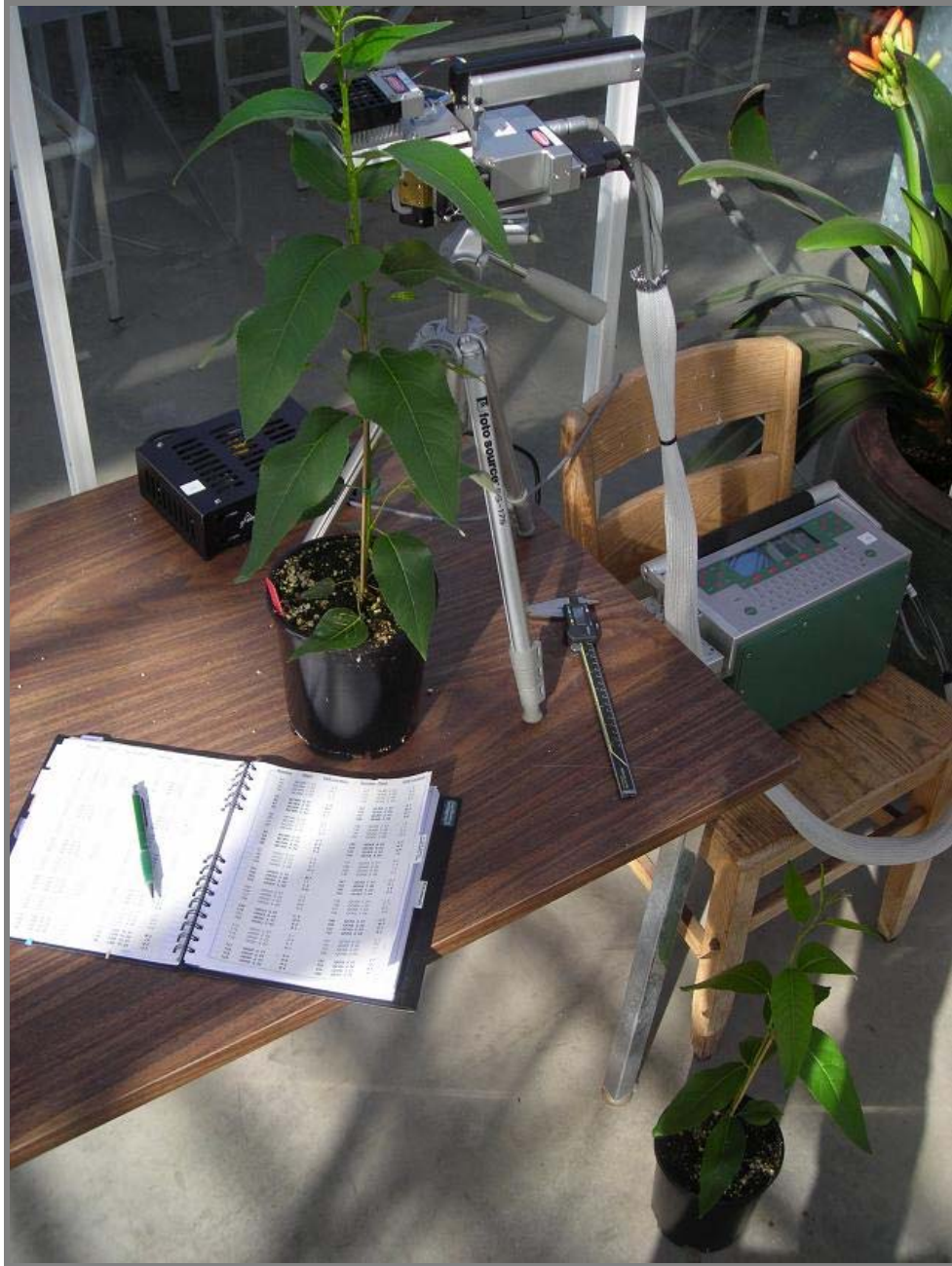
Illustration 1. Gas-exchange measurements using the LICOR 6400.
