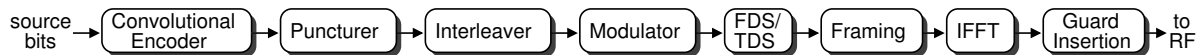
Figure 2.1: Block diagram of the MB-OFDM transmission system. FDS: frequency-domain spreading; TDS: time-domain spreading; IFFT: inverse fast Fourier transform.
