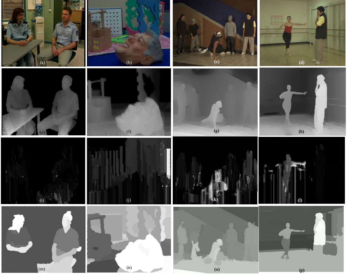
Figure 3.8 2D video sequence (a, b, c, d), recorder depth map (e, f), depth map estimated by stereo matching (g, h) estimated depth map by [12] (i, j, k, l), and estimated depth map by our approach (m, n, o, p).
