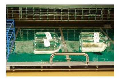
Figure 3-2 Serum bottles with resin in 100 mL solution for sorption isotherm test.
