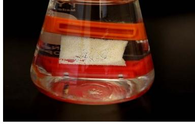
Figure 3-3 Set up for kinetics adsorption experiments of resin inside the membrane.
