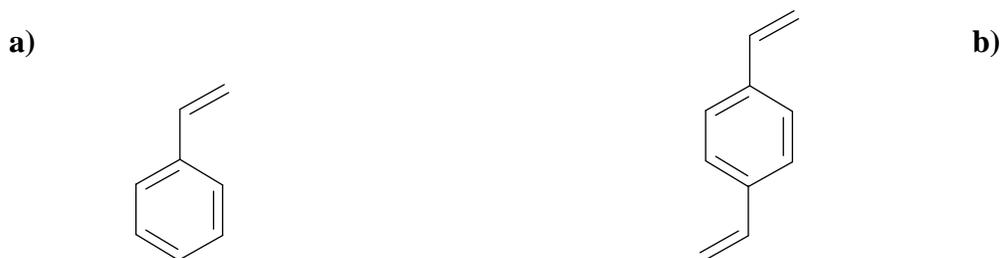
**Figure 2-2 a) Styrene (STY) and b) divinylbenzene (DVB) structures.**
