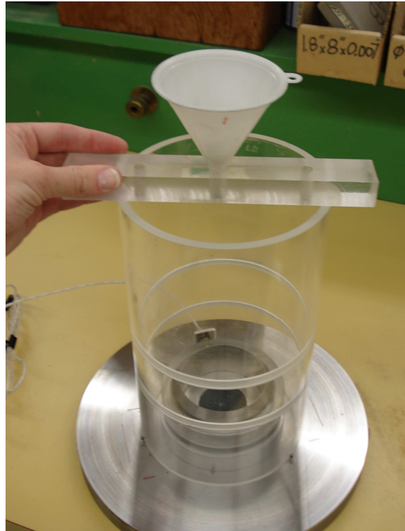
Figure 4.8. Photograph of funnel deposition with pluviation crossbar and cylinder
