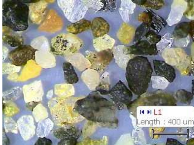
Figure 4.2. Optical microscope photograph of Fraser River sand
