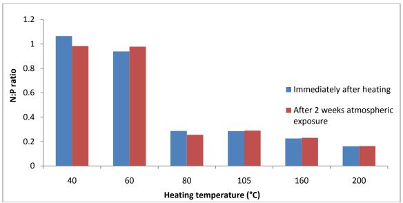
Figure 12 N:P ratio comparison of pellets immediately after heating and after 2 weeks exposure to atmospheric moisture.
