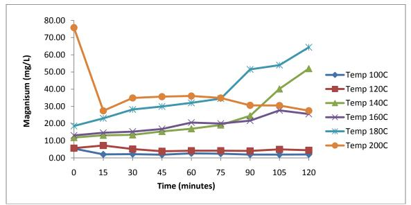
Figure 29 Magnesium concentration for Gold Bar struvite at pH 9.
