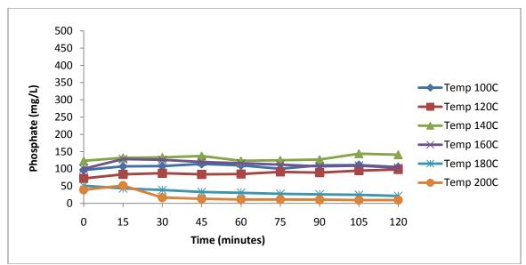
Figure 27 Orthophosphate concentration for Gold Bar struvite at pH 10.
