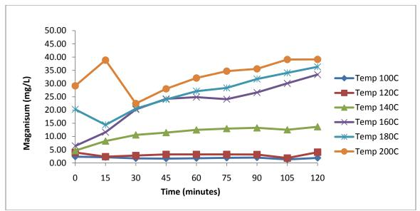
Figure 30 Magnesium concentration for Gold Bar struvite at pH 10.
