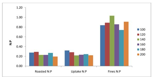
Figure 41 N:P ratios for roasted, uptake, and fine struvite. Six different roasting temperatures were used and all uptake experiments were conducted at pH 10.
