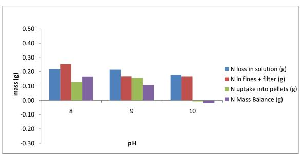
Figure D. 4 2009 nitrogen mass balance @ T=160 for pH 8,9,10
