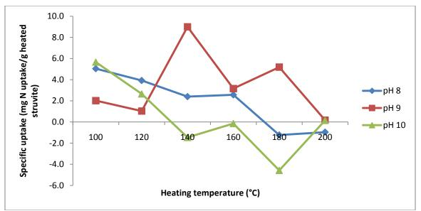
Figure 84 2009 specific uptake versus heating temperature for three pH values.
