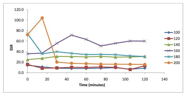
Figure 33 SSR vs. time for various temperatures at pH 10.
