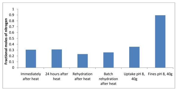
Figure 10 Effect of different environments on the nitrogen content in struvite heated at 105°C.
