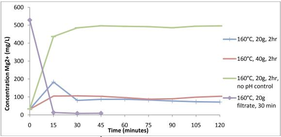
Figure 68 Effect of no pH control on Mg<sup>2+</sup> concentration.
