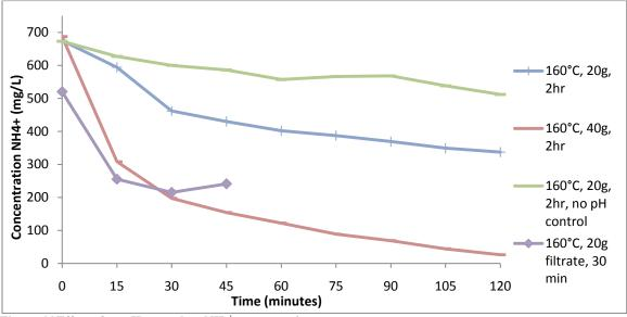
Figure 66 Effect of no pH control on NH<sub>4</sub><sup>+</sup> concentration.
