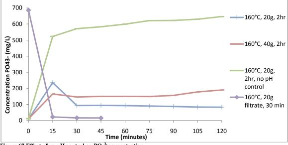
Figure 67 Effect of no pH control on PO<sub>4</sub><sup>3-</sup> concentration.
