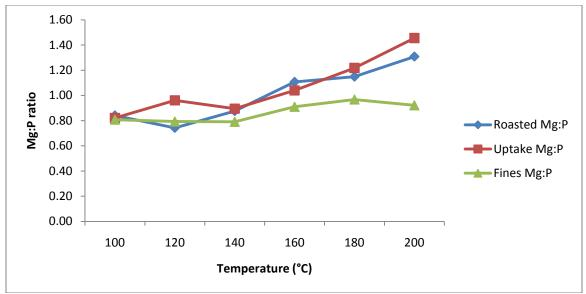
Figure 50 Mg:P ratios versus temperature for pH 8.
