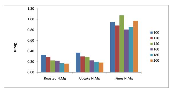
Figure 43 N:Mg ratios for roasted, uptake, and fine struvite. Six different roasting temperatures were used and all uptake experiments were conducted at pH 9.
