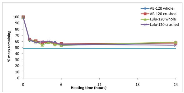
Figure 18 Percent mass remaining versus time comparing size and morphology at a heating temperature of 120°C.
