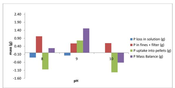
Figure D. 11 2009 phosphorus mass balance @ T=180 for pH 8,9,10
