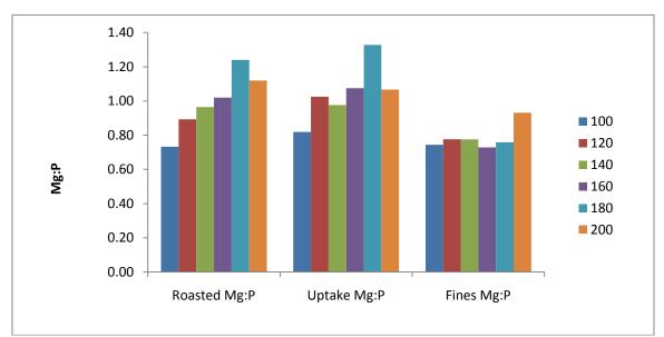
Figure 46 Mg:P ratios for roasted, uptake, and fine struvite. Six different roasting temperatures were used and all uptake experiments were conducted at pH 9.
