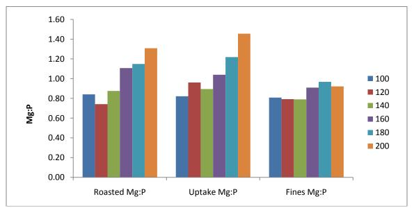
Figure 45 Mg:P ratios for roasted, uptake, and fine struvite. Six different roasting temperatures were used and all uptake experiments were conducted at pH 8.
