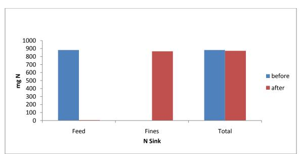
Figure 81 Nitrogen balance for 20g complete dissolution and reformation for a heating temperature of 80°C.
