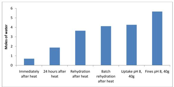
Figure 11 Effect of different environments on the water content in struvite heated at 105°C.
