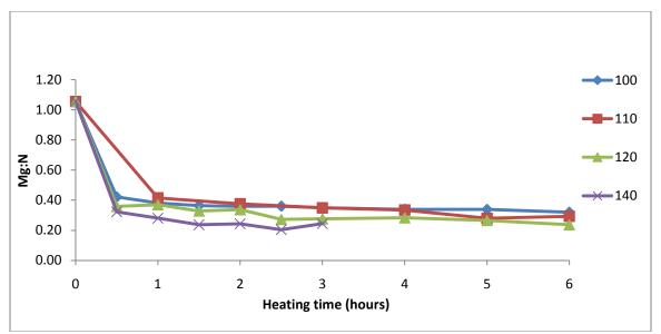
Figure 21 N:Mg vs. heating time for four temperatures.
