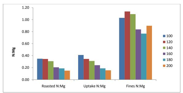
Figure 42 N:Mg ratios for roasted, uptake, and fine struvite. Six different roasting temperatures were used and all uptake experiments were conducted at pH 8.
