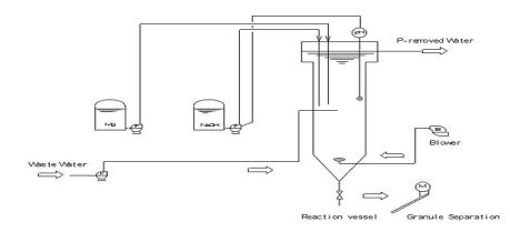
Figure 1 Struvite process diagram.
