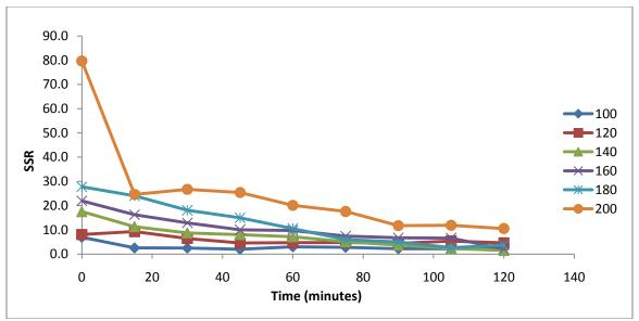
Figure 32 SSR vs. time for various temperatures at pH 9.
