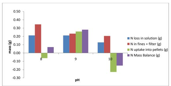
Figure D. 5 2009 nitrogen mass balance @ T=180 for pH 8,9,10
