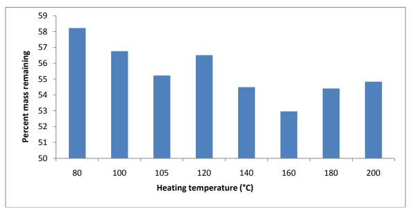
Figure 15 Percent mass remaining after 24 hours heating.
