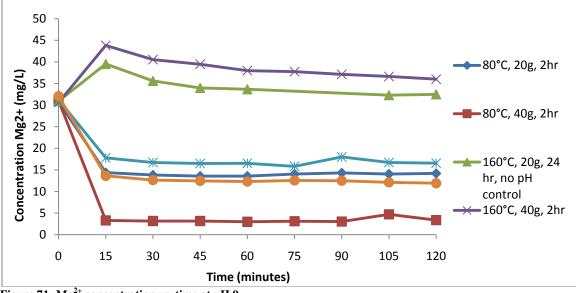
Figure 71 Mg<sup>2+</sup> concentration vs. time at pH 9.
