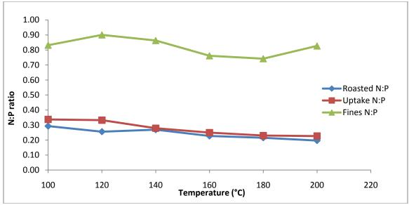
Figure 48 N:P ratios versus temperature for pH 8.
