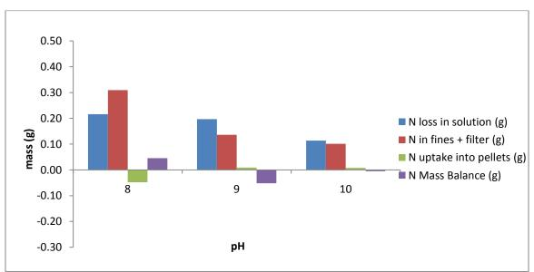
Figure D. 6 2009 nitrogen mass balance @ T=200 for pH 8,9,10
