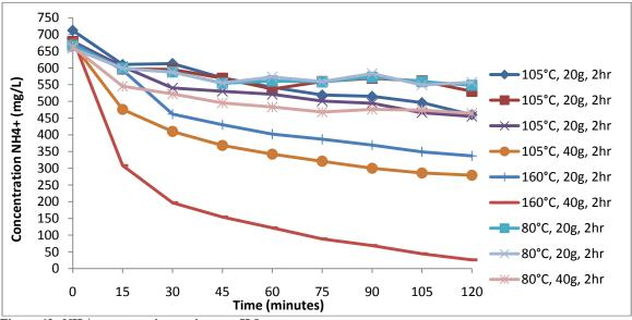
Figure 63 NH<sub>4</sub><sup>+</sup> concentration vs time at pH 8.
