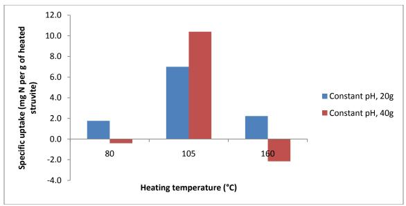
Figure 86 2010 specific uptake versus heating temperature at pH 9.
