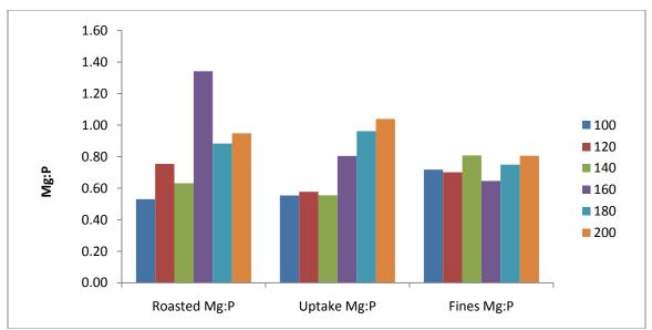
Figure 47 Mg:P ratios for roasted, uptake, and fine struvite. Six different roasting temperatures were used and all uptake experiments were conducted at pH 10.
