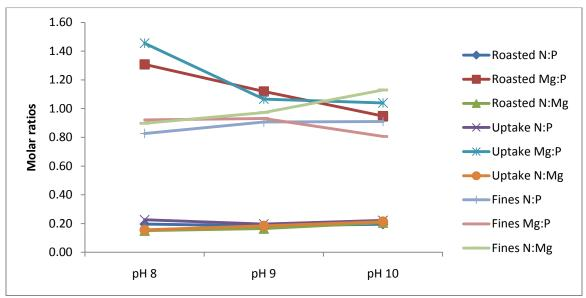
Figure 62 Solid product molar ratios vs. pH for a heating temperature of 200°C.
