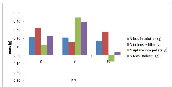
Figure D. 3 2009 nitrogen mass balance @ T=140 for pH 8,9,10
