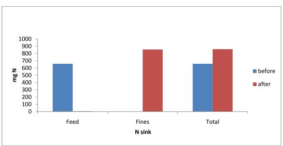
Figure 82 Nitrogen balance for 20g complete dissolution and reformation for a heating temperature of 160°C.
