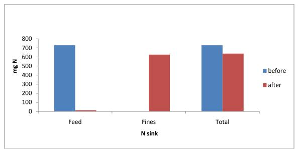
Figure 79 Nitrogen balance for 10g complete dissolution and reformation for a heating temperature of 105°C.
