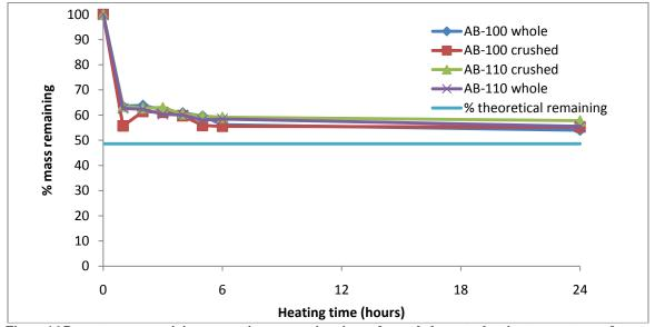
Figure 16 Percent mass remaining versus time comparing size and morphology at a heating temperature of 100°C.
