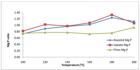
Figure 53 Mg:P ratios versus temperature for pH 9.
