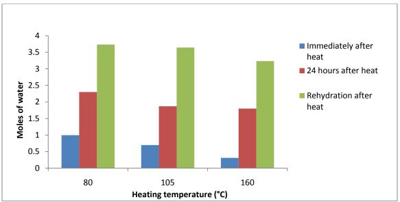
Figure 9 Effect of heating temperature on struvite water content for three different environments.
