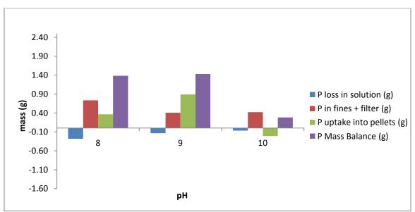
Figure D. 10 2009 phosphorus mass balance @ T=160 for pH 8,9,10
