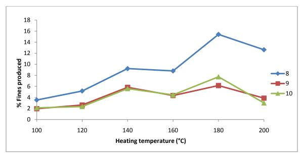
Figure 34 Percent fines produced versus isothermal heating temperature for pH 8, 9, and 10.
