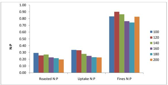
Figure 39 N:P ratios for roasted, uptake, and fine struvite. Six different roasting temperatures were used and all uptake experiments were conducted at pH 8.
