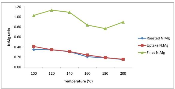
Figure 49 N:Mg ratios versus temperature for pH 8.
