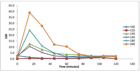
Figure 31 SSR vs. time for various temperatures at pH 8.
