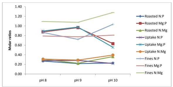
Figure 59 Solid product molar ratios vs. pH for a heating temperature of 140°C.
