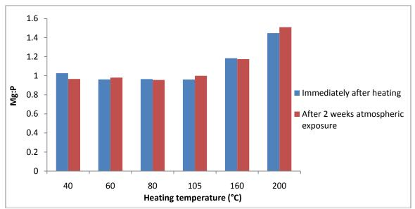
Figure 14 Mg:P ratio comparison of pellets immediately after heating and after 2 weeks exposure to atmospheric moisture.
