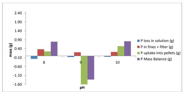
Figure D. 7 2009 phosphorus mass balance @ T=100 for pH 8,9,10
