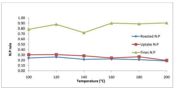
Figure 51 N:P ratios versus temperature for pH 9.
