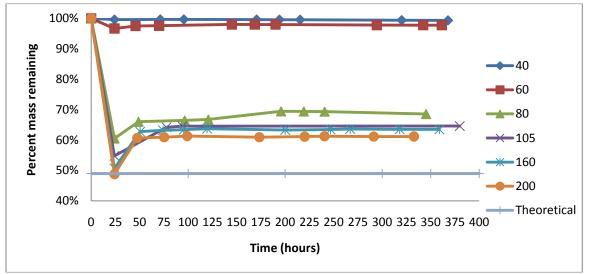
Figure 4 Percent struvite mass remaining over time for six different 24-hour heat treatments.
