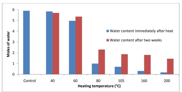
Figure 7 Water content immediately after heating compared to after two weeks exposed to the atmosphere for six different temperatures and 24 hour duration.
