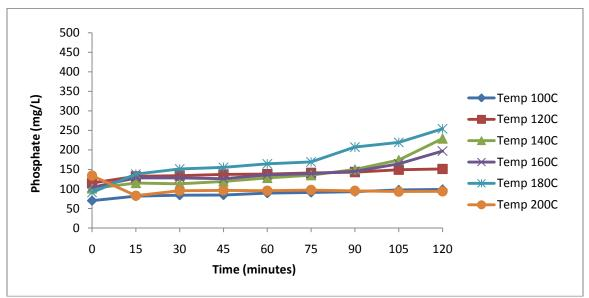
Figure 26 Orthophosphate concentration for Gold Bar struvite at pH 9.
