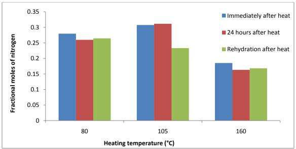
Figure 8 Effect of heating temperature on struvite nitrogen content for three different environments.
