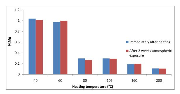
Figure 13 N:Mg ratio comparison of pellets immediately after heating and after 2 weeks exposure to atmospheric moisture.
