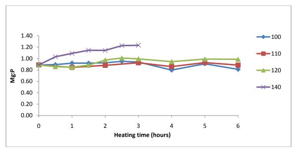
Figure 19 Mg:P vs. heating time for four temperatures.
