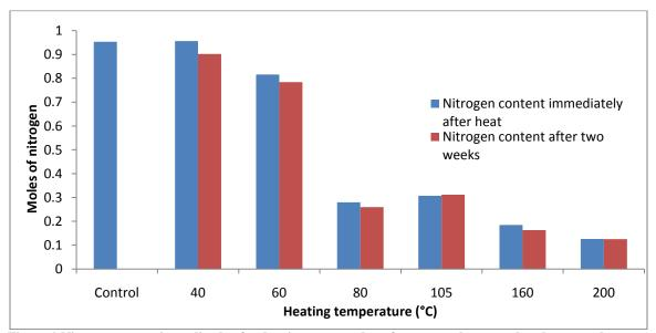
Figure 6 Nitrogen content immediately after heating compared to after two weeks exposed to the atmosphere for six different temperatures and 24 hour duration.
