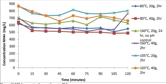
Figure 69 NH<sub>4</sub><sup>+</sup> concentration vs. time at pH 9.
