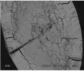
Figure 88 Heated Gold Bar struvite interior 70x.
