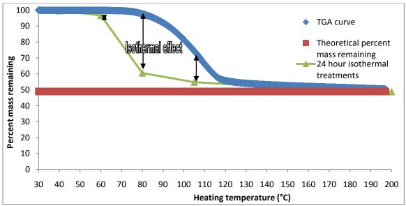
Figure 3 Struvite TGA curve – Percent mass remaining versus temperature.
