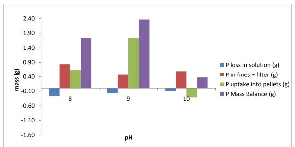
Figure D. 9 2009 phosphorus mass balance @ T=140 for pH 8,9,10
