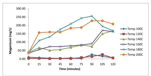
Figure 28 Magnesium concentration for Gold Bar struvite at pH 8.
