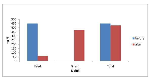
Figure 80 Nitrogen balance for 5.7g complete dissolution and reformation for a heating temperature of 160°C.
