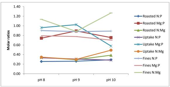
Figure 58 Solid product molar ratios vs. pH for a heating temperature of 120°C.
