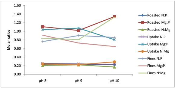
Figure 60 Solid product molar ratios vs. pH for a heating temperature of 160°C.
