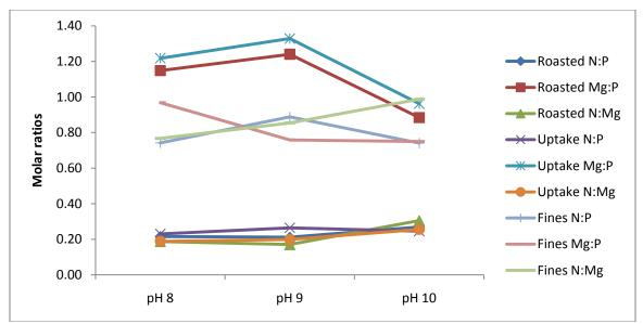
Figure 61 Solid product molar ratios vs. pH for a heating temperature of 180°C.
