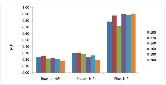
Figure 40 N:P ratios for roasted, uptake, and fine struvite. Six different roasting temperatures were used and all uptake experiments were conducted at pH 9.
