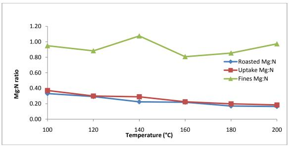
Figure 52 N:Mg ratios versus temperature for pH 9.
