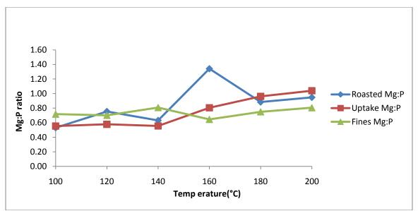
Figure 56 Mg:P ratios versus temperature for pH 10.
