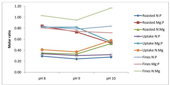
Figure 57 Solid product molar ratios vs. pH for a heating temperature of 100°C.
