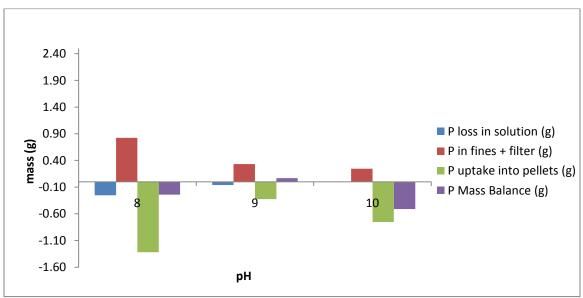
Figure D. 12 2009 phosphorus mass balance @ T=200 for pH 8,9,10
