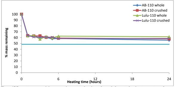
Figure 17 Percent mass remaining versus time comparing size and morphology at a heating temperature of 110°C.
