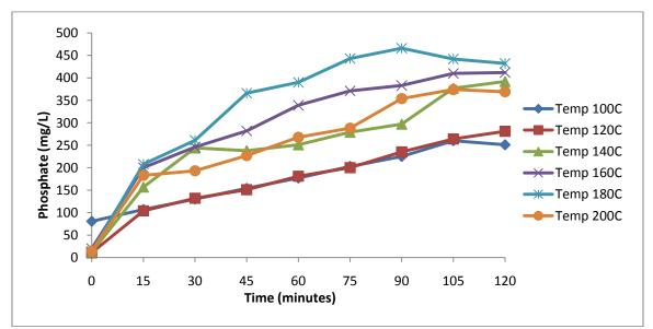
Figure 25 Orthophosphate concentration for Gold Bar struvite at pH 8.
