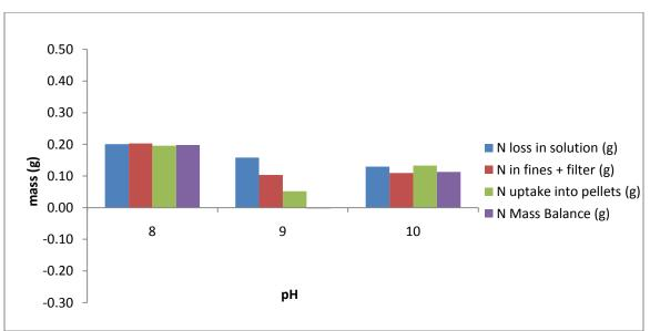
Figure D. 2 2009 nitrogen mass balance @ T=120 for pH 8,9,10
