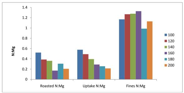
Figure 44 N:Mg ratios for roasted, uptake, and fine struvite. Six different roasting temperatures were used and all uptake experiments were conducted at pH 10.
