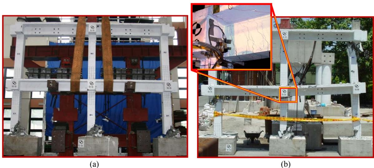
**Figure 5-17. Comparison of failure modes during Test2; a) specimen MCFS; b) specimen HCFS**
