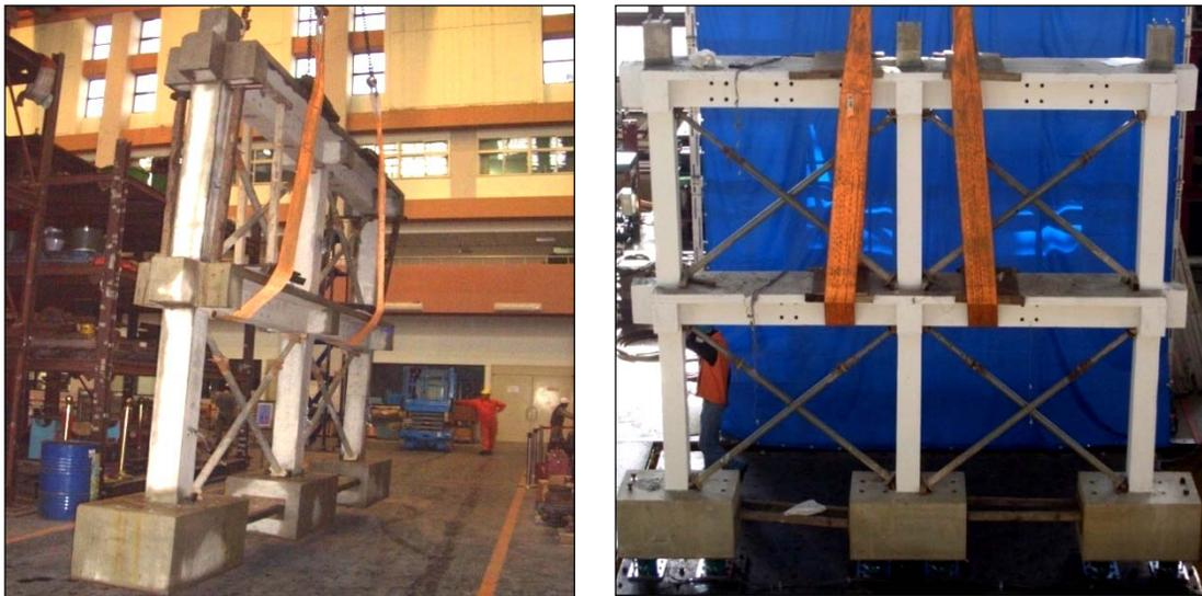
**Figure 3-5. Locating the specimens on the shaking table**
