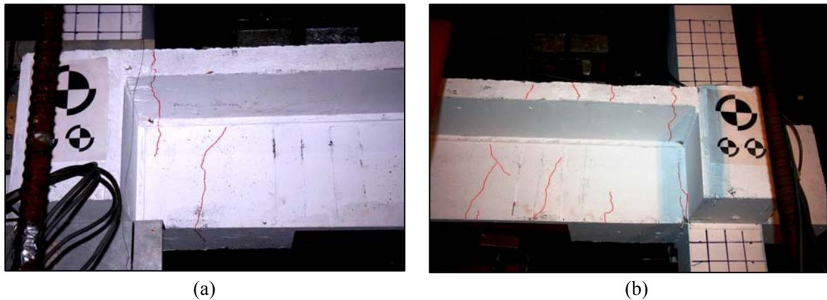
**Figure 4-24. Cracks in beams after Test1; a) near joint C1; b) near joint A1**
