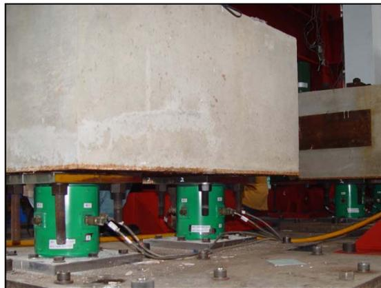
**Figure B-1. Connection of load cells to footings and shaking table**
