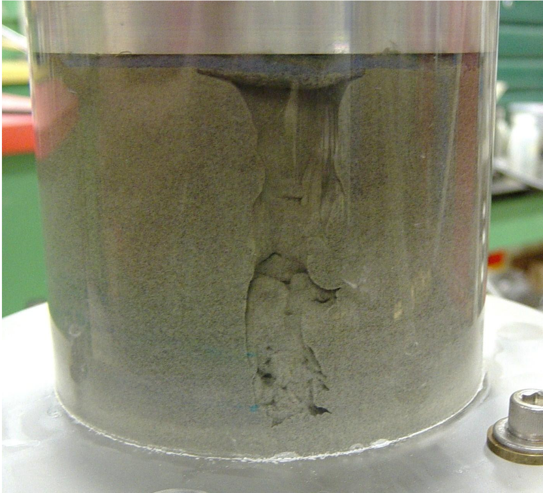
Figure D8 Soil specimen after test D-W2-T6 ( AOS/D_{85} \approx 3.7 )
