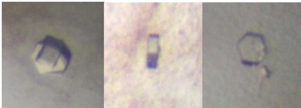
Figure 6.6 Examples of crystals grown from solutions containing FL-gelsolin and GsnVHH9. The precipitant used was 33.0%(v/v) PEG600, 200 mM imidazole malate buffer, pH 5.5.
