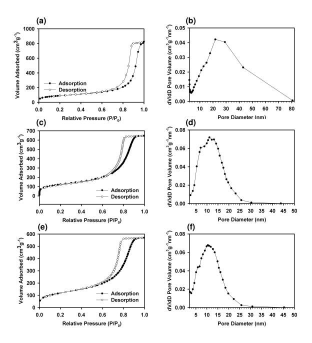
**Figure 3-9.** Nitrogen adsorption data for mesoporous silica films prepared by acid hydrolysis of **Comp3**. (a) N<sub>2</sub> isotherm for **CNMS3-H<sub>2</sub>SO<sub>4</sub>**. (b) BJH pore size distribution for **CNMS3-H<sub>2</sub>SO<sub>4</sub>**. (c) N<sub>2</sub> isotherm for **CNMS3-HCl**. (d) BJH pore size distribution for **CNMS3-HCl**. (e) N<sub>2</sub> isotherm for **CNMS3-HCl-Cal**. (f) BJH pore size distribution for **CNMS3-HCl-Cal**.
