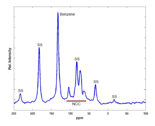
**Figure B-3.** <sup>13</sup>C CP/MAS solid-state NMR of **Bz-CNMO**. Peak labeled benzene corresponds to the phenylene bridge of the organosilica. Peaks labeled SS are spinning sidebands, artifacts from spinning the rotor that are often large for aromatic samples. Small additional peaks that may come from residual NCC or glucose are also present.
