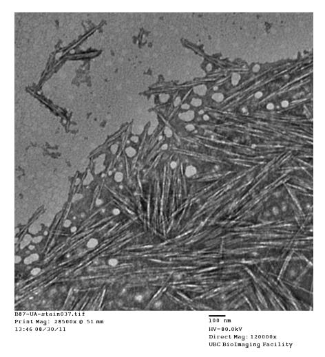
**Figure A-2.** TEM micrograph of negatively stained NCC template at higher magnification.
