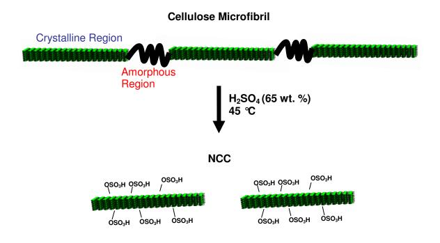
Figure 1-7. Schematic illustration of NCC synthesis by sulfuric acid hydrolysis.
