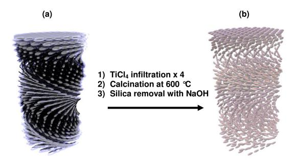
**Scheme 4-1.** Schematic representation of the synthesis of chiral nematic mesoporous titania. (a) Chiral nematic mesoporous silica used as a hard template. (b) Chiral nematic mesoporous titania replica.
