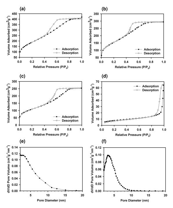
**Figure 2-8.** Nitrogen adsorption data for selected calcined samples (a)  $N_2$  isotherm for **CNMS1**. (b)  $N_2$  isotherm for **CNMS3**. (c)  $N_2$  isotherm for **MS3-pH2.0**. (d)  $N_2$  isotherm for **MS3-pH12.5**. (e) BJH pore size distribution for **CNMS1**. (f) BJH pore size distribution for **CNMS6**.
