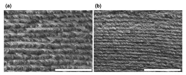
**Figure 2-9.** SEM comparison of chiral nematic film before and after calcination. (a) Cross-sectional micrograph of **Comp2** (scale bar =  $2 \mu m$ ). (b) Cross-sectional micrograph of **CNMS2** (scale bar =  $2 \mu m$ ).
