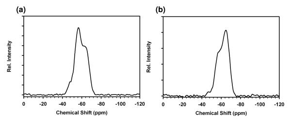
Figure 3-3. <sup>29</sup>Si CP/MAS solid-state NMR spectra of (a) Et-Comp3 and (b) Et-CNMO3.
