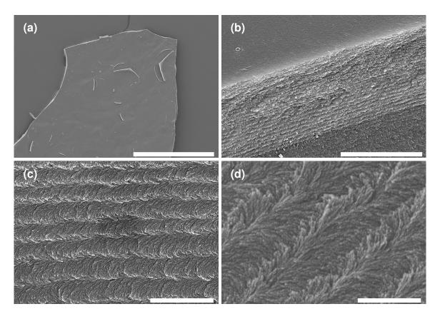
**Figure 5-8.** SEM micrographs of **CNMC3**. (a) Top view of film at low magnification (scale bar =  $500 \, \mu m$ ). (b) Side view at fracture (scale bar =  $5 \, \mu m$ ). (c) Cross-sectional view of film (scale bar =  $2 \, \mu m$ ). (d) High magnification image of cross-section (scale bar =  $500 \, nm$ ).
