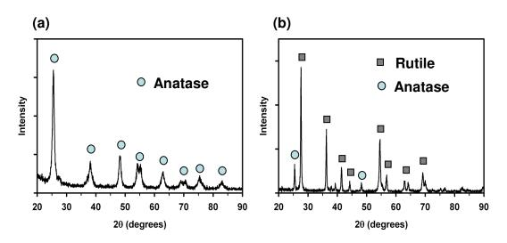
**Figure 4-3.** PXRD patterns for (a) **Ti-Acid** and (b) **Ti-Control**. **Ti-Cal** is not shown but gives a pattern virtually identical to **Ti-Acid**.
