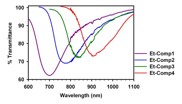
Figure 3-1. UV-Vis/NIR spectra of Et-Comp1-4.
