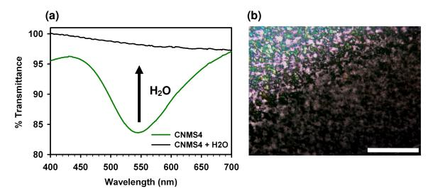
**Figure 2-15.** Water infiltration of **CNMS4**. (a) UV-Vis spectra of **CNMS4** before and after the addition of water. (b) POM micrograph of **CNMS4** after the addition of water (scale bar =  $200 \mu m$ ). The green area in the top-left region of the image is still dry.
