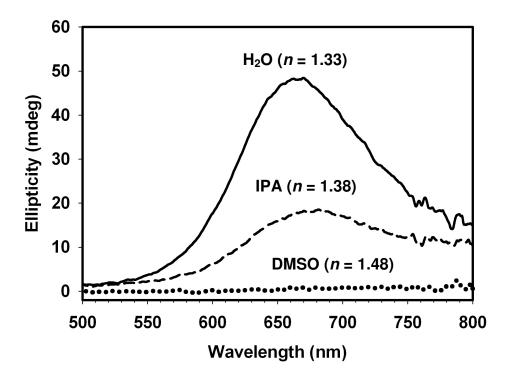
**Figure 2-16**. Circular dichroism spectra of **CNMS5** after infiltration with different liquids.
