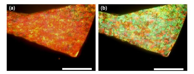
**Figure 4-7.** (a) POM micrographs **Ti-Acid**. (a) Micrograph of a dry **Ti-Acid** film (scale bar =  $400 \mu m$ ). (b) Micrograph of the same film after wetting with ethanol (scale bar =  $400 \mu m$ ).
