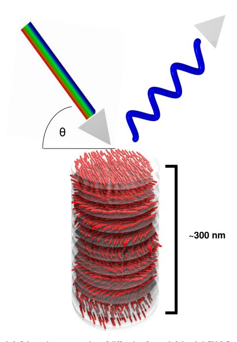
**Figure 1-4.** Schematic representation of diffraction from a left-handed CN-LC with P of  $\sim 300$  nm. Left-handed circularly polarized blue light is selectively reflected while the remaining incoming light is transmitted.
