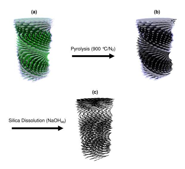
**Scheme 5-1.** Conversion of a chiral nematic NCC/silica composite film to chiral nematic mesoporous carbon. (a) NCC/silica composite film. (b) Carbon/silica composite film obtained after pyrolysis of (a) at 900  $^{\circ}$ C under an N<sub>2</sub> atmosphere. (c) Mesoporous carbon obtained after the treatment of (b) with 2M NaOH.
