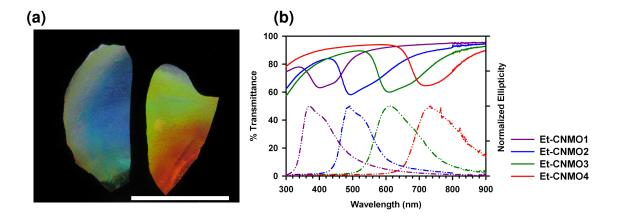
**Figure 3-5**. Optical characterization of Et-CNMO films. (a) Photograph of **Et-CNMO2** (left) and **Et-CNMO3** (right, scale bar = 18 mm). (b) UV-Vis/NIR (solid lines) and CD spectra (dashed lines) of **Et-CNMO1-4**.
