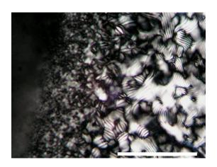
**Figure 2-1.** POM micrograph of a drop taken from an NCC/TMOS mixture during evaporation on a glass slide. The right side of the image (closer to the edge of the drop) displays a fingerprint texture indicative of a chiral nematic LC phase (scale bar =  $100 \mu m$ ).
