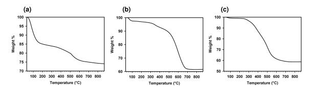
**Figure B-1.** TGA run under air for different organosilica samples: (a) **Me-CNMO**, (b) **Bz-CNMO**, and (c) **Hex-CNMO**.
