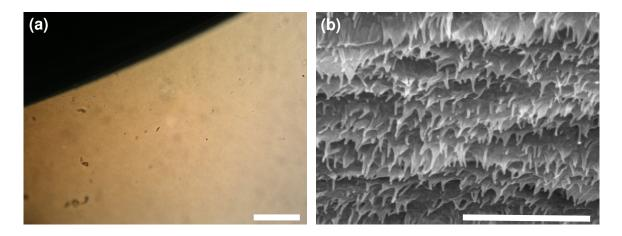
**Figure 2-5**. Disruption of chiral nematic ordering by the addition of HCl. (a) POM micrograph of **Comp3-pH2.0** (scale bar =  $100 \mu m$ ). (b) Cross-sectional SEM micrograph of **Comp3-pH2.0** (scale bar =  $1 \mu m$ ).
