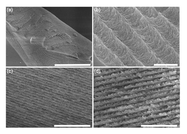
**Figure 3-6.** SEM images of Et-CNMO films. (a) Top view of fracture for **Et-CNMO3** (scale bar = 30  $\mu$ m). (b) High magnification micrograph of **Et-CNMO3** (scale bar = 1  $\mu$ m). (c) Cross-sectional micrograph of **Et-CNMO1** (scale bar = 2  $\mu$ m). (d) Cross-sectional micrograph of **Et-CNMO4** (scale bar = 2  $\mu$ m).
