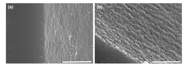
**Figure 5-9.** SEM micrographs of MC1 and CNMC2. (a) Top view of fracture of MC1 film (scale bar = 1  $\mu$ m). (b) Top view of fracture of CNMC2 film (scale bar = 1  $\mu$ m).
