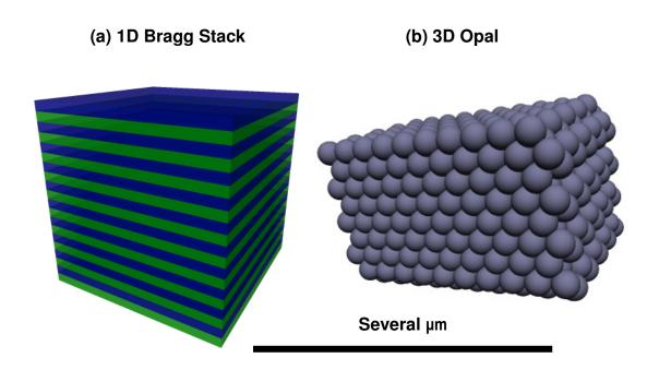
**Figure 1-2.** Representative examples of photonic crystal structures. (a) The different coloured layers represent materials with different refractive indices. (b) The opal structure consists of spheres arranged in an fcc lattice.
