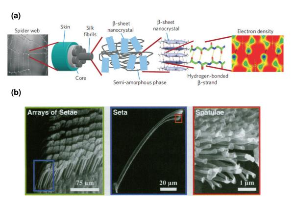
**Figure 1-1.** Examples of hierarchically structured biological nanomaterials. (a) The nanostructure of spider silk gives it its incredible strength. (b) The nanostructured setae present on gecko feet give them remarkable adhesive properties. (a) was reproduced in part by permission from Macmillan Publishers Ltd: Nature Materials, <sup>[19]</sup> copyright 2010. (b) was reproduced in part from reference 26. Copyright 2005 National Academy of Sciences, USA.
