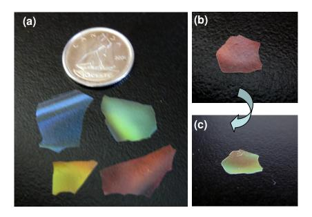
**Figure 2-12.** Photographs of iridescent silica films. (a) Silica films **CNMS3-6**. The dime is included for scale (d = 18 mm). (b) Photograph of **CNMS6** taken at normal incidence. (c) Photograph of **CNMS6** taken at oblique incidence.
