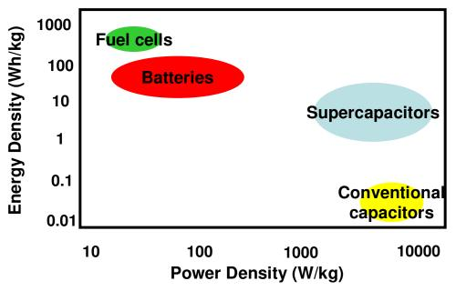
Figure 1-12. Ragone plot comparing performance of different energy storage devices.
