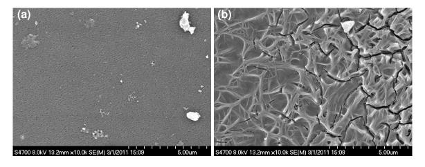
**Figure C-2.** SEM images showing the surface of **Ti-Acid** films. (a) Image showing a region without any surface crust. (b) Image showing a region with a surface crust.
