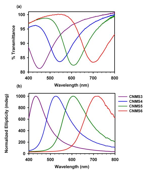
**Figure 2-13.** Optical characterization of iridescent silica films **CNMS3-6**. (a) UV-Vis spectra of **CNMS3-6**. (b) CD spectra of **CNMS3-6**.
