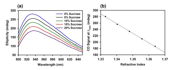
**Figure 3-13.** (a) CD spectra for **Et-CNMO2** after soaking with different aqueous sucrose solutions. (b) Plot of max CD signal vs. refractive index based on the spectra shown in (a).
