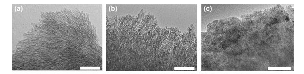
**Figure 5-7.** TEM micrographs of porous carbon samples. (a) TEM micrograph of **CNMC3**. (b) TEM micrograph of **MC3-pH2.0**. (c) TEM micrograph of **MC1**. Scale bars all = 200 nm.
