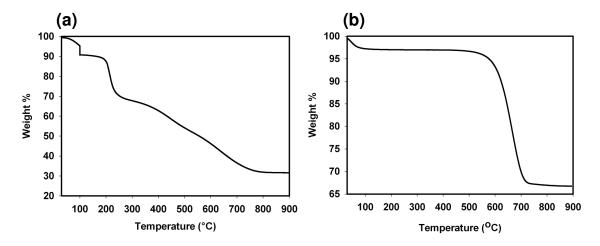
**Figure 5-1.** (a) TGA of **Comp3**. (b) TGA of **Comp3** after carbonization at 900 °C. Both samples were run under air.
