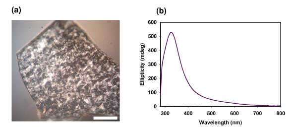
**Figure 5-10.** Optical characterization of silica templated by **CNMC3**. (a) POM micrograph (scale bar =  $200 \mu m$ ). (b) CD spectrum.
