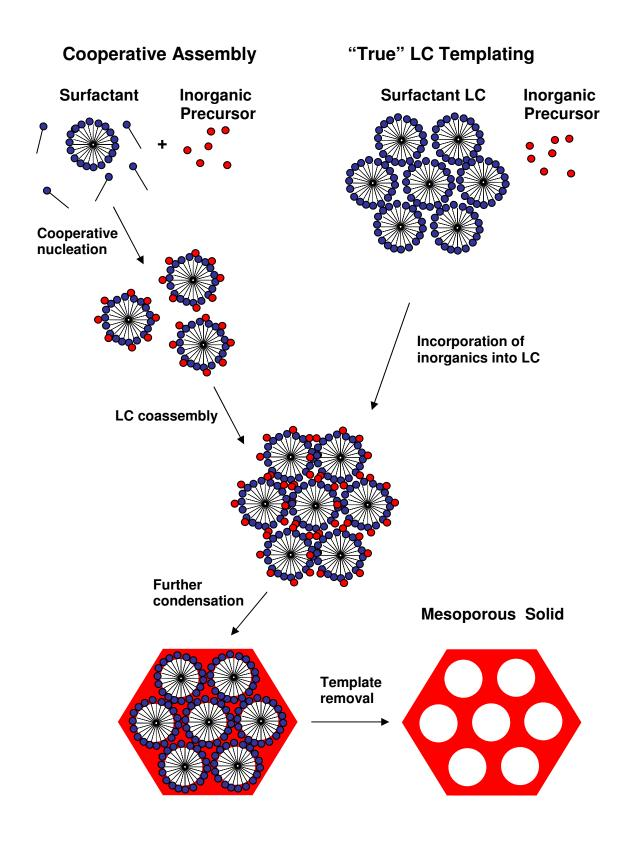
**Figure 1-9**. Synthesis of ordered mesoporous materials by cooperative self-assembly and "true" liquid crystal templating pathways.
