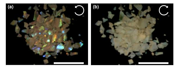
**Figure 4-5.** Circular polarized iridescence of **Ti-Acid**. (a) **Ti-Acid** photographed using a left-handed circular polarizing filter (scale bar = 2 cm). (b) **Ti-Acid** photographed using a right-handed circular polarizing filter (scale bar = 2 cm).
