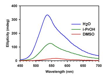
Figure 3-12. CD spectra of Et-CNMO2 after wetting with different liquids.
