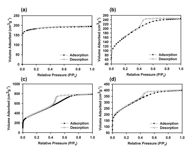
**Figure 5-5.** Nitrogen adsorption isotherms for selected carbon samples. (a)  $N_2$  isotherm measured for **MC1**. (b)  $N_2$  isotherm measured for **CNMC2**. (c)  $N_2$  isotherm measured for **CNMC3**. (d)  $N_2$  isotherm measured for **CNMC5**.
