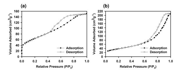
Figure 4-4. N<sub>2</sub> adsorption isotherms for mesoporous titania (a) Ti-Cal and (b)Ti-Acid.
