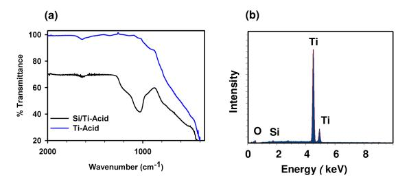
**Figure 4-2.** Data showing the removal of SiO<sub>2</sub> by NaOH treatment of SiO<sub>2</sub>/TiO<sub>2</sub> composite. (a) IR spectra before (**Si/Ti-Acid**) and after (**Ti-Acid**) NaOH treatment of SiO<sub>2</sub>/TiO<sub>2</sub> composite. (b) EDX spectrum of **Ti-Acid**.
