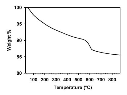
Figure C-1. TGA of Ti-Acid run under air.
