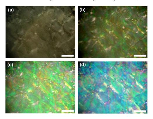
**Figure 3-11.** POM micrographs of Et-CNMO2 taken at different time points after wetting with acetone. (a) **Et-CNMO2** immediately after wetting with acetone. (b) **Et-CNMO2** 15 seconds after wetting with acetone. (c) **Et-CNMO2** 17 seconds after wetting with acetone. (d) **Et-CNMO2** 30 seconds after wetting with acetone. All scale bars =  $200 \, \mu m$ .
