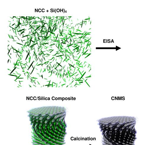
**Scheme 2-1.** Outline of the synthesis of chiral nematic NCC/silica composite films and chiral nematic mesoporous silica (CNMS).
