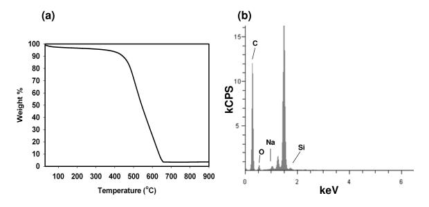
**Figure 5-3.** TGA and EDX characterization of mesoporous carbon. (a) TGA of **CNMC3** (10 °C/min, air). (b) EDX spectrum of **CNMC3**. The two unlabeled peaks at 1.25 and 1.5 keV correspond to Mg and Al found in the SEM stub.
