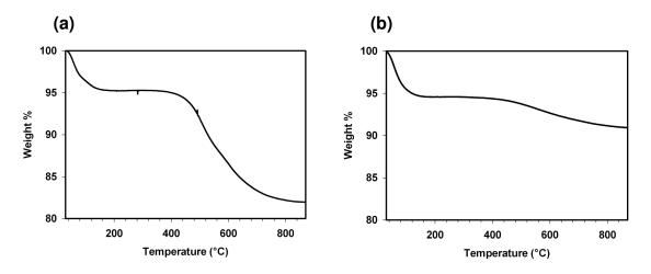
Figure 3-4. TGA of (a) Et-CNMO3 and (b) CNMS3- H<sub>2</sub>SO<sub>4</sub>.
