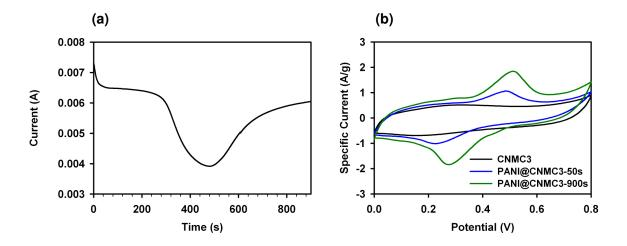
**Figure 5-16.** Electrochemical characterization of selected **PANI@CNMC3** samples. (a) Current vs. time curve during a 900 s PANI electropolymerization carried out at 0.8 V vs. Ag/AgCl. (b) CV curves for selected samples obtained at a scan rate of 2 mV/s (all CVs were run with a three electrode setup, potential is vs. Ag/AgCl).
