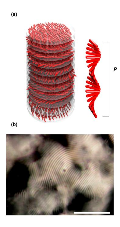
**Figure 1-3.** (a) Schematic representation of a CN-LC. Discrete layers are shown (left) to illustrate the structure, although in a real CN-LC the rotation of the nematic director is continuous. The right side shows the orientation of the nematic director in each layer as it makes a full  $360^{\circ}$  rotation corresponding to the distance P. (b) Polarized optical micrograph of a CN-LC showing characteristic fingerprint texture (scale bar =  $30 \,\mu\text{m}$ ).
