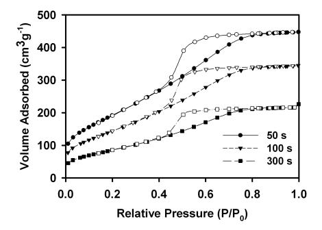
**Figure 5-15.** Nitrogen adsorption isotherms for **PANI@CNMC3** electropolymerized for 50, 100, and 300 seconds.
