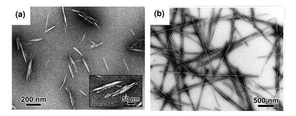
**Figure 1-6**. TEM micrographs of negatively stained NCC. (a) NCC prepared by sulfuric acid hydrolysis of cotton. (b) NCC prepared by sulfuric acid hydrolysis of tunicate. Reproduced in part with permission from reference 50. Copyright 2008 American Chemical Society.
