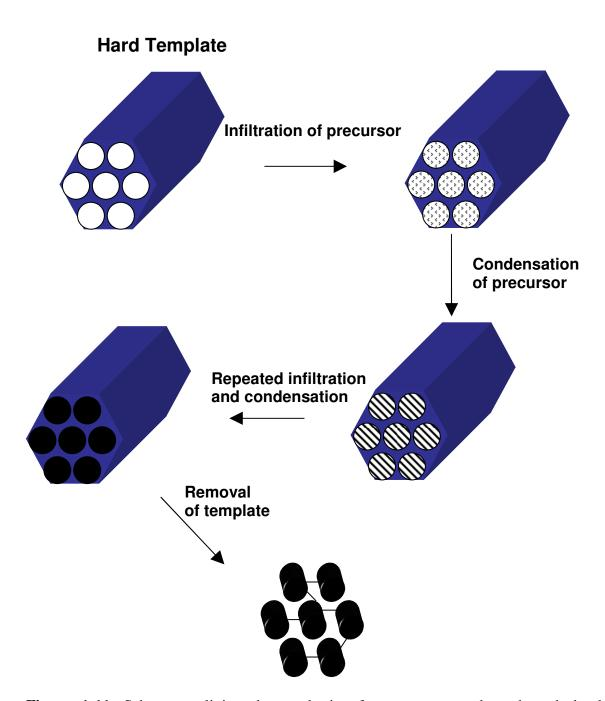
**Figure 1-11.** Scheme outlining the synthesis of mesoporous carbon through hard templating.
