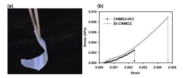
**Figure 3-10**. Improved flexibility of Et-CNMO films. (a) Photograph of a film from sample **Et-CNMO2** being bent with tweezers. (b) Comparison of stress-strain curves obtained from tensile testing of mesoporous silica (**CNMS3-HCl**) and organosilica (**Et-CNMO2**) samples.
