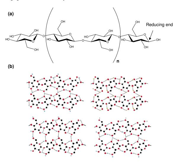
**Figure 1-5.** Molecular structure of cellulose. (a) Chemical structure of an individual cellulose polymer chain. (b) Possible hydrogen-bonding patterns for cellulose I found in plants. (b) was reproduced in part with permission from reference 47. Copyright 2004 American Chemical Society.
