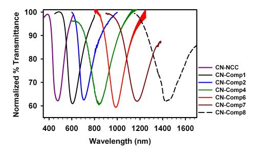
**Figure 2-4.** UV-Vis spectra for chiral nematic NCC and selected NCC/silica composite films.
