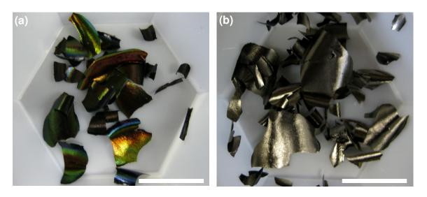
**Figure 5-2.** Photographs of carbon films before and after the removal of silica. (a) Carbon/silica composite films derived from **Comp3** (scale bar = 2 cm). (b) Mesoporous carbon sample **CNMC3** (scale bar = 2 cm).
