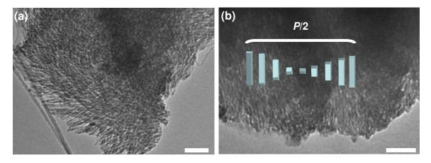
**Figure 2-10.** TEM micrographs of **CNMS3**. (a) View looking down the helical axis of a film fragment (scale bar = 100 nm). (b) Film fragment with the helical axis in the plane of the image as indicated (scale bar = 100 nm).
