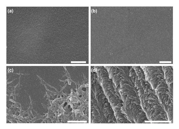
**Figure 5-13.** SEM micrographs of selected samples. (a) Top surface of a **CNMC3** film before PANI deposition. (b) Top surface of a **PANI@CNMC3** film after 100 second electropolymerization. (c) Top surface of a **PANI@CNMC3** film after 300 second electropolymerization. (d) Edge of **PANI@CNMC3** film after 300 second electropolymerization. Scale bars all = 500 nm.
