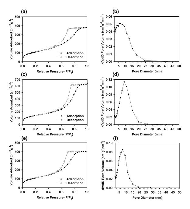
**Figure 3-7**. Nitrogen adsorption data for selected ethylene-bridged mesoporous organosilica samples. (a) N<sub>2</sub> isotherm for **Et-CNMO1**. (b) BJH pore size distribution for **Et-CNMO3**. (c) N<sub>2</sub> isotherm for **Et-CNMO3**. (d) BJH pore size distribution for **Et-CNMO3**. (e) N<sub>2</sub> isotherm for **Et-CNMO3-Cal**. (f) BJH pore size distribution for **Et-CNMO3-Cal**.
