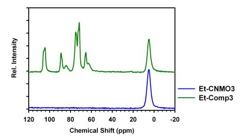
**Figure 3-2**. <sup>13</sup>C CP/MAS solid-state NMR of ethylene-bridged organosilica before (green) and after (blue) the removal of NCC.
