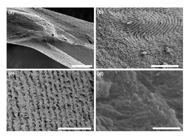
**Figure 2-7.** SEM images of calcined silica **CNMS2**. (a) Top view looking down the edge of a fractured film (scale bar =  $10 \mu m$ ). (b) Cross-sectional micrograph of film showing repeating structure with fingerprint defect (scale bar =  $10 \mu m$ ). (c) Cross-sectional view at higher magnification (scale bar =  $2 \mu m$ ). (d) High magnification micrograph looking down the chiral nematic helical axis (scale bar = 200 nm).
