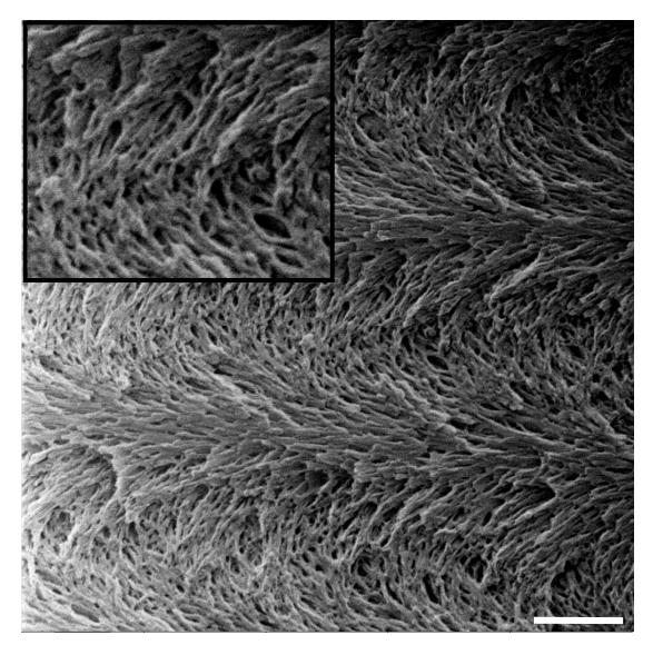
**Figure 3-8**. Helium ion micrograph of **Et-CNMO3** (scale bar = 200 nm). The inset shows a blown-up section taken from the middle of the image.
