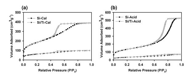
**Figure 4-1.** N<sub>2</sub> adsorption isotherms before and after TiO<sub>2</sub> loading. (a) Isotherms for **Si-Cal** and the corresponding silica/titania composite obtained after the final TiCl<sub>4</sub> loading step and calcination at 600 °C. (b) Isotherms for **Si-Acid** and the corresponding
