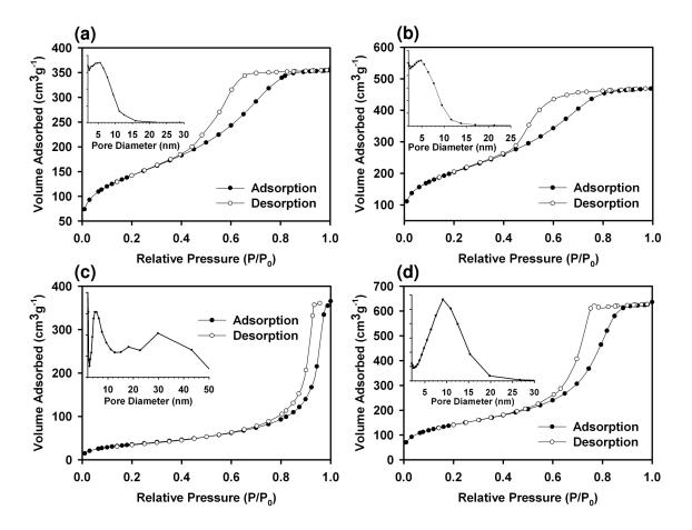
**Figure 3-16.**  $N_2$  adsorption data for organosilica samples with different bridging groups. (a)  $N_2$  adsorption isotherm and BJH pore size distribution (inset) for **Me-CNMO**. (b)  $N_2$  adsorption isotherm and BJH pore size distribution (inset) for **Bz-CNMO**. (c)  $N_2$  adsorption isotherm and BJH pore size distribution (inset) for **Hex-MO**. (d)  $N_2$  adsorption isotherm and BJH pore size distribution (inset) for **Et-CNMO3**.
