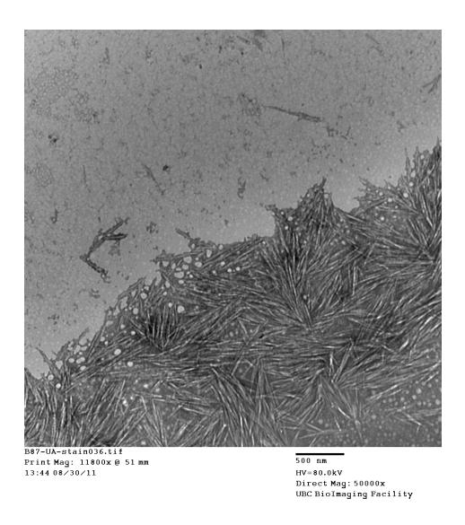
Figure A-1. TEM micrograph of negatively stained NCC template.
