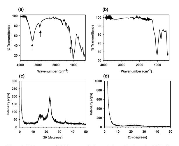
**Figure 2-6.** IR spectra and PXRD patterns before and after calcination of an NCC-silica composite film. (a) IR spectrum of **Comp1**. Arrows indicate characteristic NCC peaks (O-H, C-H, and C-C stretching modes, respectively, from left to right). (b) IR spectrum of **CNMS1**. (c) PXRD pattern of Comp1. (d) PXRD pattern for **CNMS1**.
