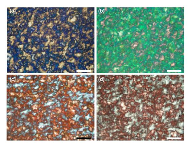
**Figure 2-11.** POM micrographs of chiral nematic silica films **CNMS3-CNMS6** (a-d respectively, all scale bars =  $100 \mu m$ ).
