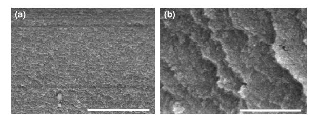
**Figure 5-11.** SEM micrographs of silica templated by **CNMC3**. (a) Cross-sectional view (scale bar =  $2 \mu m$ ). (b) Cross-sectional view at higher magnification (scale bar = 500 nm).
