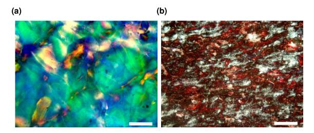
**Figure 2-3.** (a) POM micrograph of a free-standing chiral nematic NCC film (**CN-NCC**, scale bar =  $100 \ \mu m$ ). (b) POM micrograph of free-standing NCC/silica composite film **Comp3** (scale bar =  $100 \ \mu m$ ).
