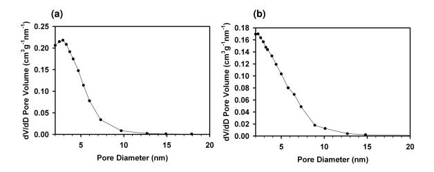
**Figure 5-6.** (a) BJH pore size distribution for **CNMC3**. (b) BJH pore size distribution for **MC3-pH2.0**.
