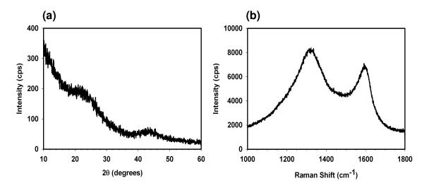
**Figure 5-4.** Spectroscopic characterization of mesoporous carbon. (a) PXRD pattern of **CNMC3**. (b) Raman spectrum of **CNMC3**.
