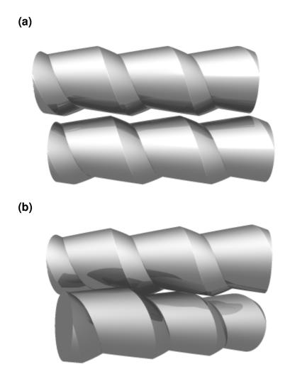
**Figure 1-8**. Different packing arrangements of screw-shaped rods. (a) Parallel arrangement. (b) Chiral arrangement, which can facilitate closer packing.
