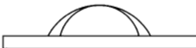
Figure 4.8: Diagram of the spherical calotte morphology suggested by Ciobanu et al 43 . In this morphology the inner core is exposed to the outside environment.
