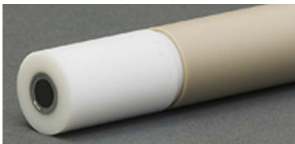
Figure 3.2 Rotating ring disk electrode assembly
