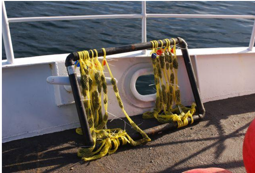
Figure 4.1. Mussels in net socks, attached to a plastic frame, in preparation for subtidal exposure.
