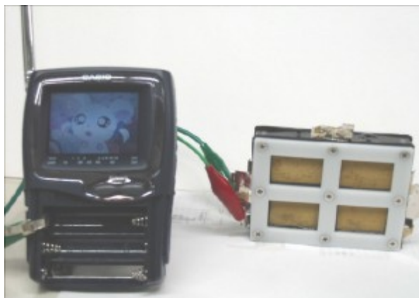
Figure 14. DBFC stack operating under passive and ambient conditions powering a small television. The anolyte composition was 5 wt% \text{NaBH}_4 – 20 wt% \text{NaOH} , and the Ni powder to Pd/ C to Nafion ® anode ratio was 0.75:0.3:0.1 with a 20 \text{ mg cm}^{-2} metal loading. Reprinted with permission from [80], Copyright 2008, Elsevier.
