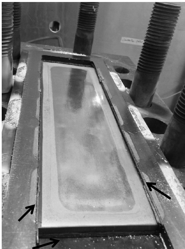
Figure 8.6: Pd/Ag Membrane Installed on Bottom Flange after Experiment no.3. Arrows indicate locations of gasket under the membrane and strips used on sides to fill gaps. They also indicate where feed by-passing is suspected to have occurred.
