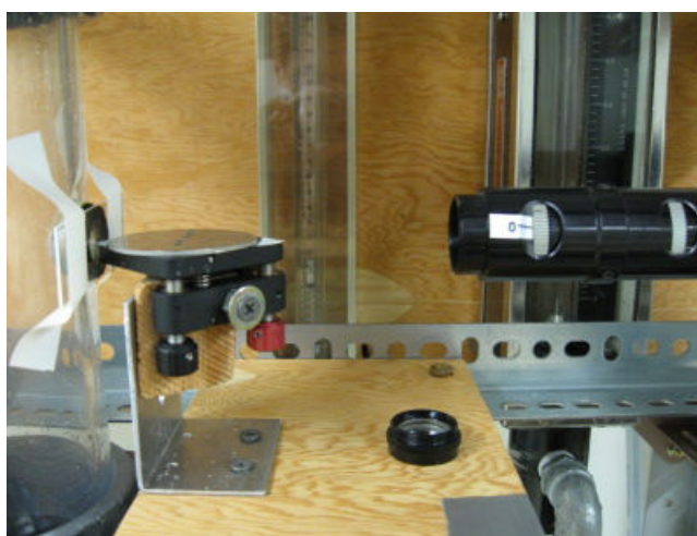
Figure 4.34 Photo of the sessile drop measurement system. Lenses are at 1 \times magnification, 90 cm away from the drops
