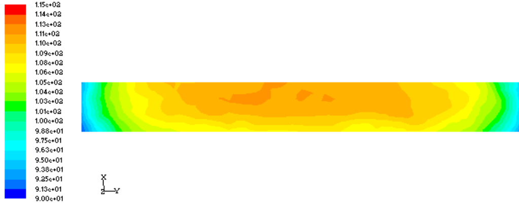
Fig. A.7. UV irradiance ( \text{W}/\text{m}^2 ) computed by the CFD simulation on the quartz plate above the catalyst-coated slides.
