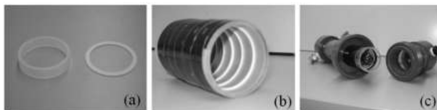
Fig. 6.2. TiO 2 -coated annular reactor with repeated ribs: (a) photocatalyst-coated tube piece and PTFE washer, (b) coated glass pieces and PTFE washers put together forming a ribbed tube, (c) ribbed tube fitted in the PVC structure.
