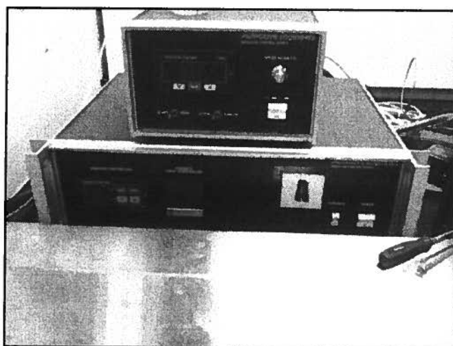
Figure 21 Temperature control (bottom unit) and stirrer control (top unit) for Autoclave Engineers reactor
