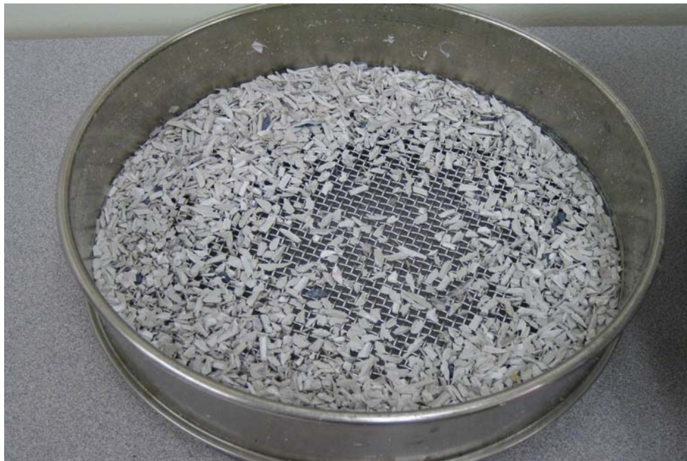
Figure 2.5 E-waste after mechanical shaking prior to weighing for particle size distribution analysis.
