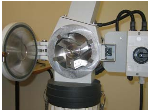
Figure 2.4 Inside of Retsch grinder SM100
