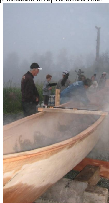
Figure 59: Steaming of T'aa canoe, Kaay, Haida Gwaii, 2008.
