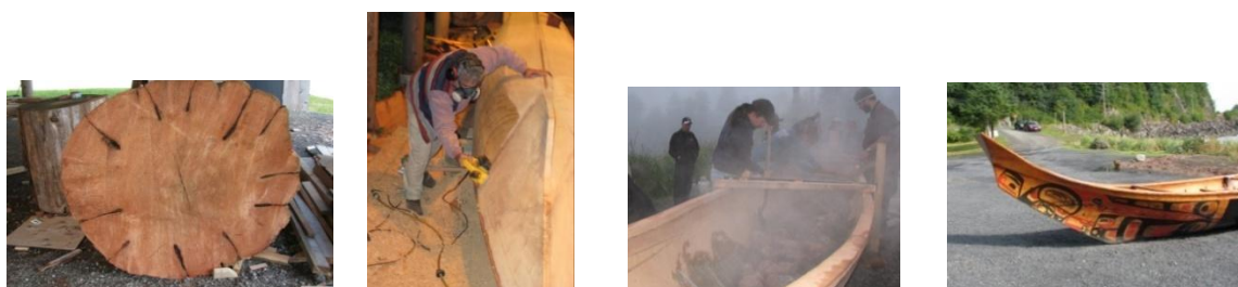
Figure 56: (L-R) Full log before shaping; Guujaaw sanding hull, HHC, Haida Gwaii, 2007; Steaming T’aa; T’aa resting on beach at Kaay, Haida Gwaii, 2008.
