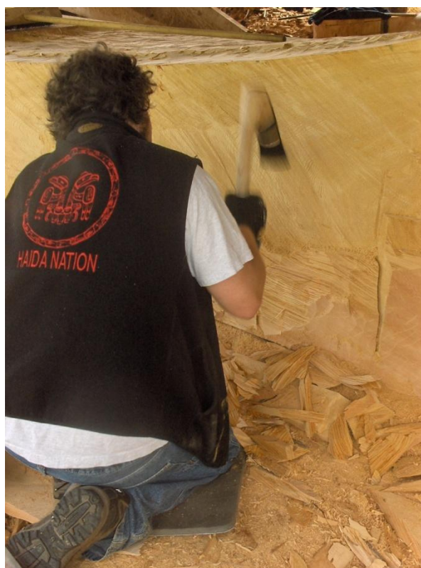
Figure 67: Jaalen Edenshaw adzing the hull of T'aa, HHC, Haida Gwaii, 2007.
