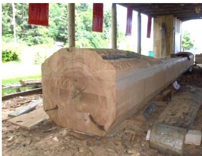
Figure 50: Early stages of shaping cedar log into canoe, HHC, Haida Gwaii, 2007.
