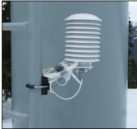
Figure 2.3: UBC temperature and relative humidity sensor (UBC3) within a radiation shield and its attachment to the ski lift tower ladder.
