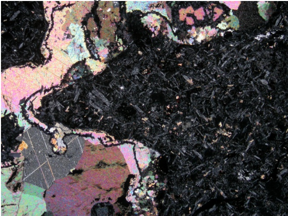
Large calcite-filled amygdale within altered cpx and plag in groundmass. Photo 9328, XPL 2x magnification, FOV = 7 mm.
