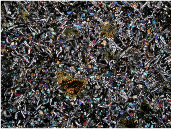
Green chlorite-filled amygdules, unaltered plag and cpx in the groundmass. Photo 9384, XPL 2x magnification, 7 mm.
