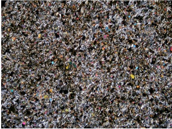
Fresh, unaltered groundmass of plag, cpx, and opaque minerals. Photo 1251, XPL 2x magnification, FOV = 7 mm.
