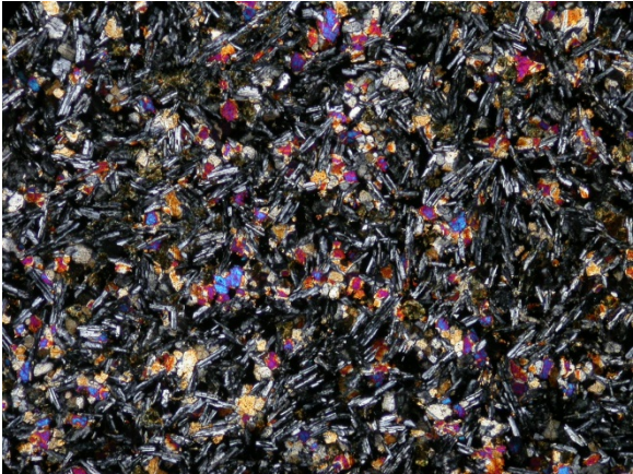
Cpx and plag in the groundmass with minor chlorite alteration. Photo 1242, XPL 5x magnification, FOV = 3 mm.
