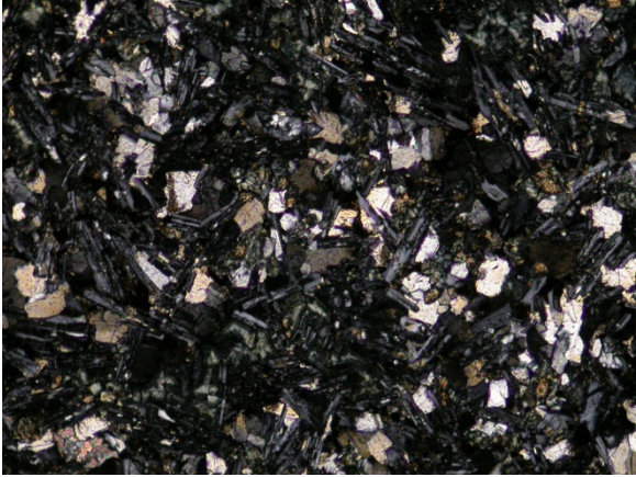
Cpx and plag in the groundmass with minor opaque minerals. Photo 9362, XPL 10x magnification, FOV = 1.5 mm.
