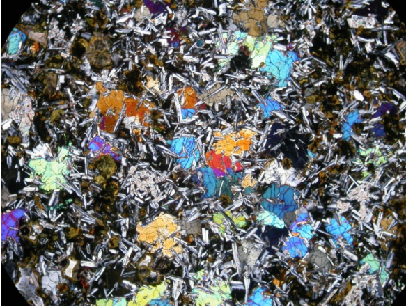
Ophitic cpx intergrown around plag, with green-brown chlorite-filled amygdules. Photo 9151, XPL 2x magnification, FOV = 7 mm.
