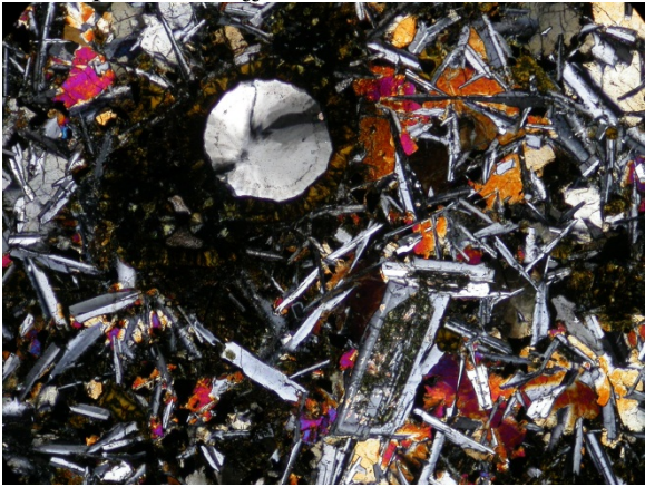
Chalcidony nodule with chlorite rim amongst plag and cpx in the groundmass. Photo 9392, XPL 5x magnification, FOV = 3 mm.
