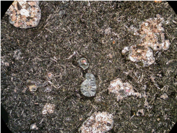
Altered basalt with chlorite- and calcite-filled amygdules, primary plag and cpx groundmass. Photo 9158, XPL 2x magnification, FOV = 7 mm.
