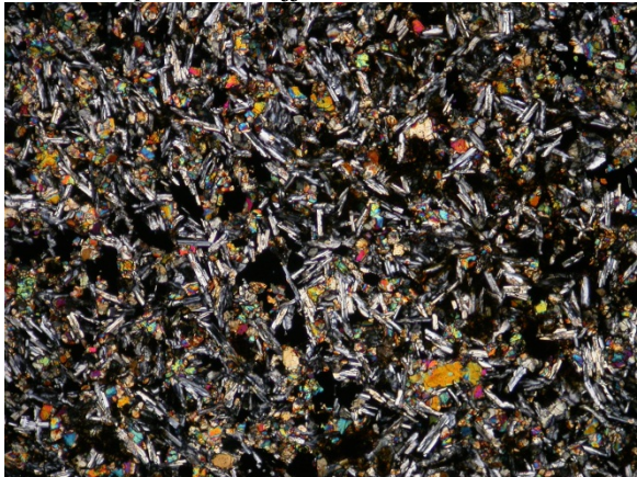
Cpx, plag, and opaque minerals in the groundmass. Photo 9380, XPL 5x magnification, FOV = 3 mm.
