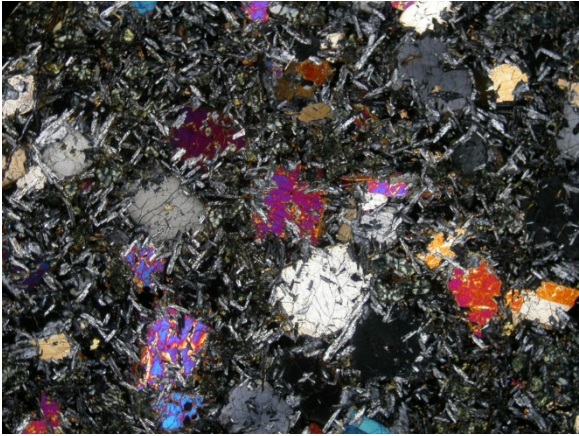
Ophitic cpx with plag in the groundmass and minor chlorite alteration. Photo 1237, 2x magnification, FOV = 7 mm.
