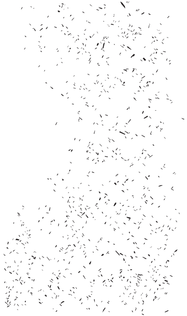
Figure C4 Thin section scan and polygon outlines of plagioclase in sample 11RAT TD129D. Left) Thin section scan of sample in crossed-polarized light (26 x 46 mm). Right) Binary (black and white images) of 912 polygon outlines of plagioclase crystals.
