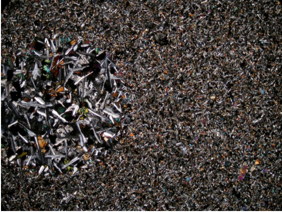
Clot of coarse-grained cpx/plag amongst groundmass. Photo 0575, XPL 2x magnification, FOV = 7mm.
