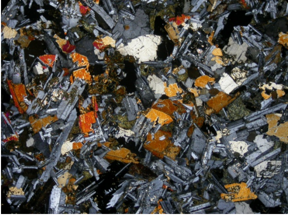
Coarse-grained cpx and plag in the groundmass. Photo 1235, XPL 2x magnification, FOV = 7 mm.
