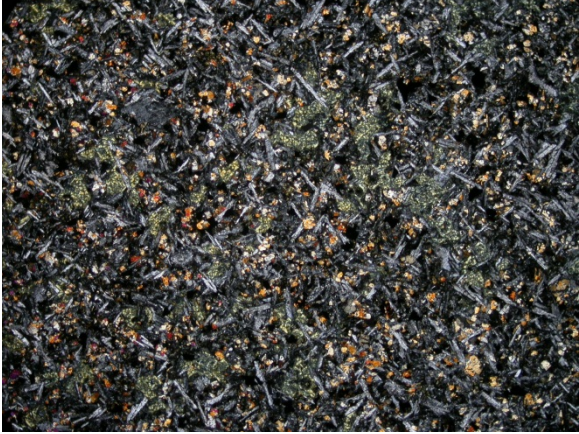
Cpx and plag in the groundmass with interspersed chlorite alteration. Photo 0584, XPL 2x magnification, FOV = 7 mm.
