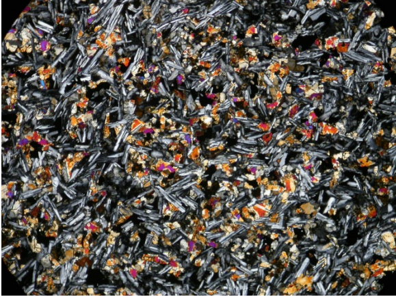
Homogeneous groundmass of cpx, plag, and opaque minerals. Photo 9164, XPL 5x magnification, FOV = 3 mm.
