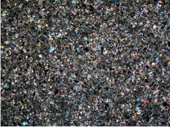
Fine-grained plag, cpx, and opaque minerals in the groundmass. Photo 0367, XPL 2x magnification, FOV = 7 mm.
