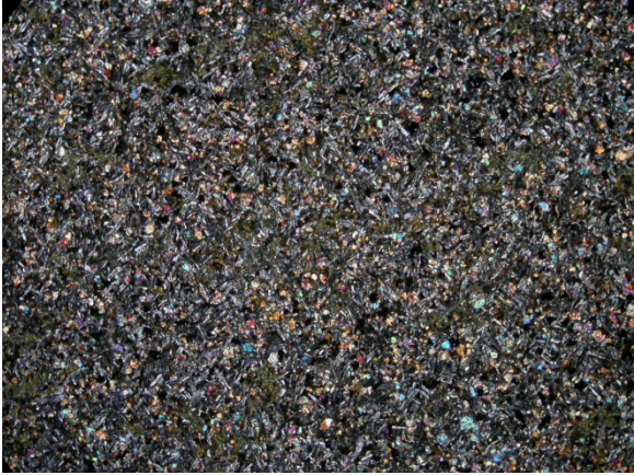
Plag and cpx in the groundmass with chlorite alteration. Photo 0359, XPL 2x magnification, FOV = 7 mm.
