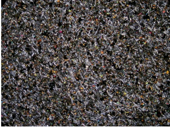
Cpx, plag, and opaque minerals in the groundmass. Photo 1240, XPL 2x magnification, FOV = 7 mm.
