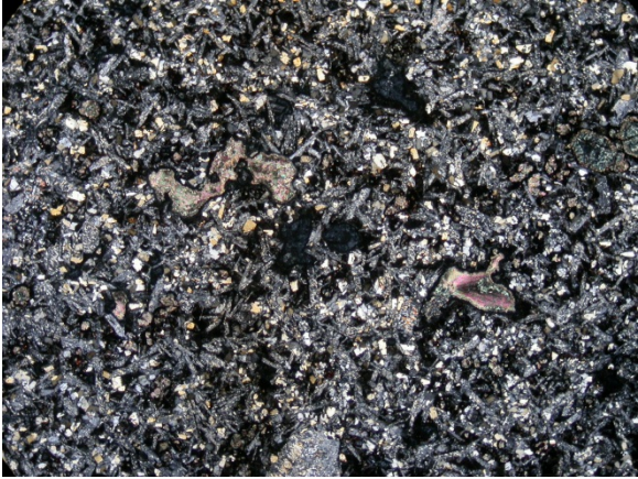
Plag and cpx in the groundmass with calcite-filled amygdules. Photo 1191, XPL 2x magnification, FOV = 7 mm.
