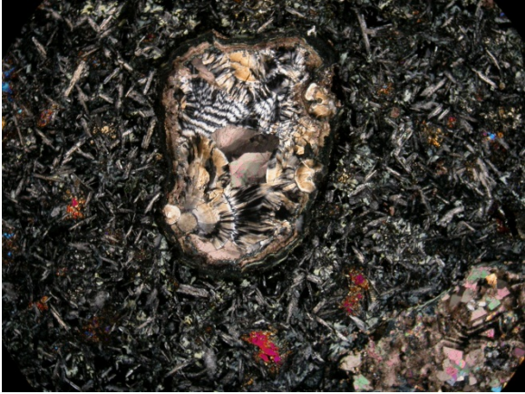
Calcite- and quartz-filled amygdule with plag and cpx in groundmass. Photo 9160, XPL 2x magnification, FOV = 7 mm.
