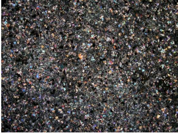
Fine-grained plag, cpx, and opaque minerals in the groundmass. Photo 0358, XPL 2x magnification, FOV = 7 mm.
