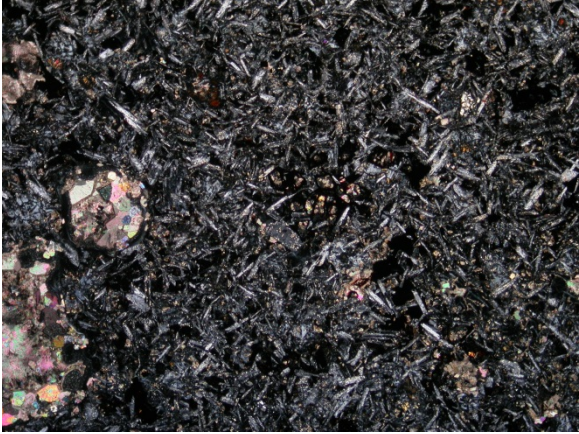
Calcite-filled amygdules and groundmass of plag and cpx. Photo 9214, XPL 2x magnification, FOV = 7 mm.
