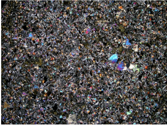
Plag and cpx in the groundmass with cpx phenocrysts. Photo 0572, XPL 2x magnification, FOV = 7 mm.
