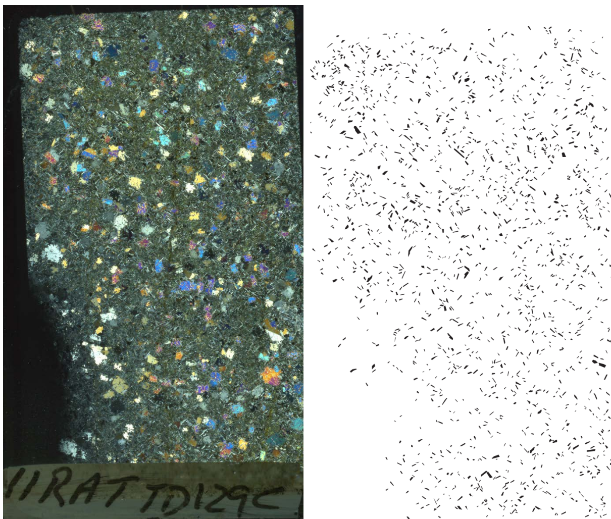
Figure C3 Thin section scan and polygon outlines of plagioclase in sample 11RAT TD129C. Left) Thin section scan of sample in crossed-polarized light (26 x 46 mm). Right) Binary (black and white images) of 1,701 polygon outlines of plagioclase crystals.
