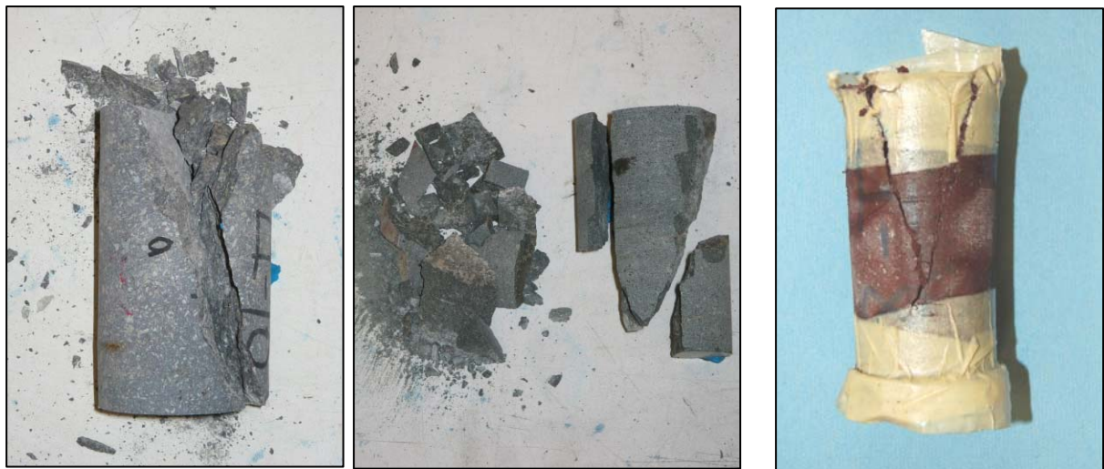
Figure 3.23. Shear failure of samples after failure subject to uniaxial and triaxial loading.
