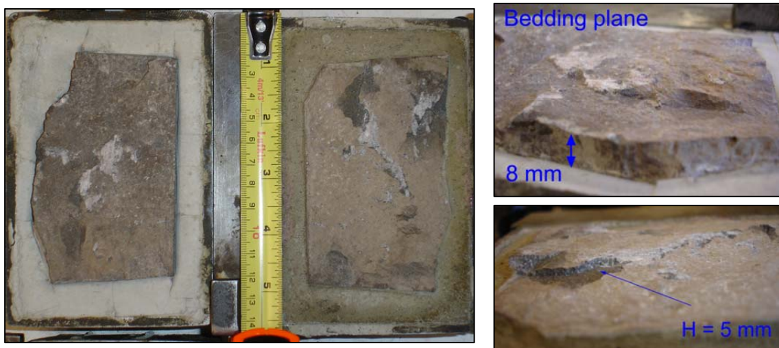
Figure 3.26. Detailed pictures obtained from the rough surface of the principal joint set (JS1).
