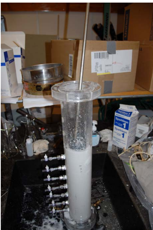
Figure A10.8 – Packing method
