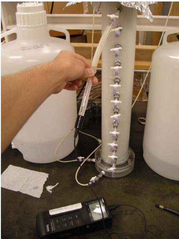
Figure A10.12 – Method of obtaining pH samples without oxygen ingress
