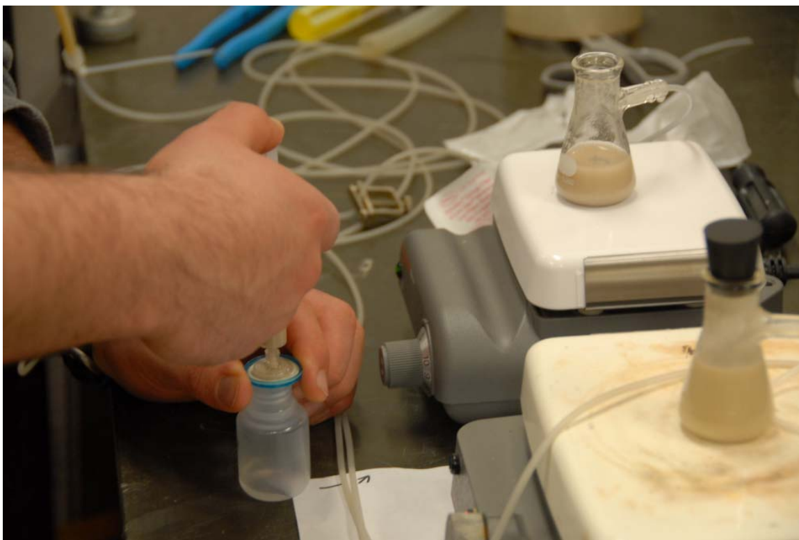
Figure A4.4 – Filtration of sample with 0.22 \mu\text{m} syringe filter
