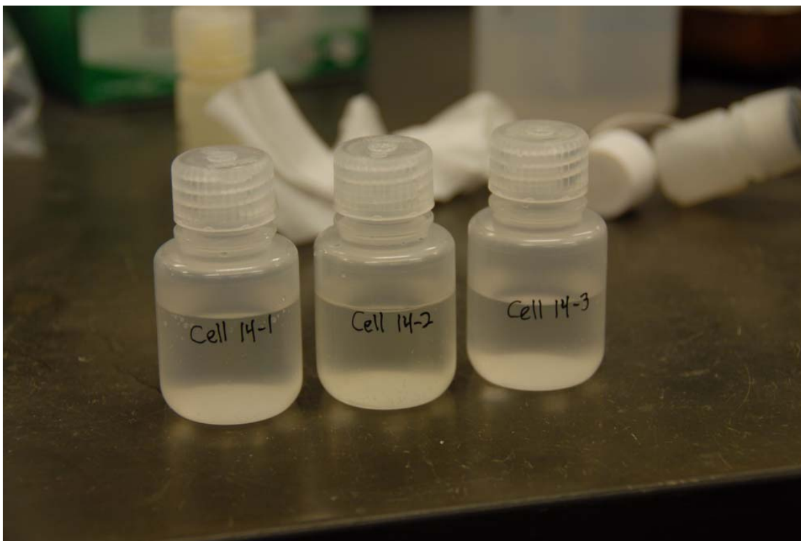
Figure A4.5 – Filtered, acidified samples ready to be stored at 4°C
