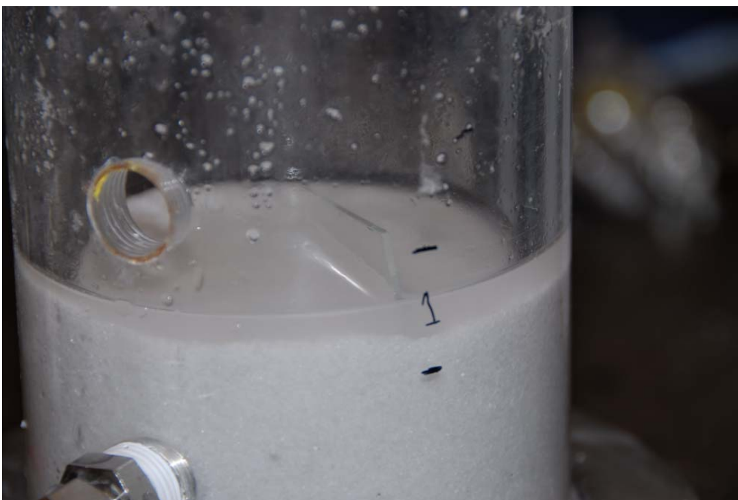
Figure A10.7 – One of the glass plates installed in the column, which proved to be useless as negligible crystals precipitated on it
