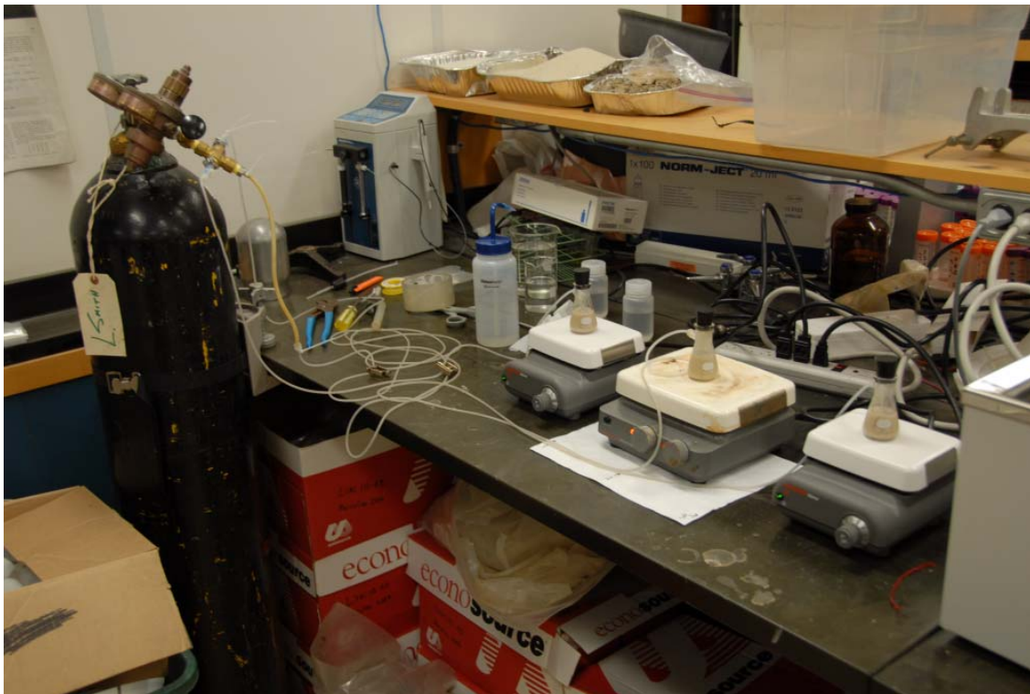
Figure A4.2 – Samples being degassed with nitrogen gas
