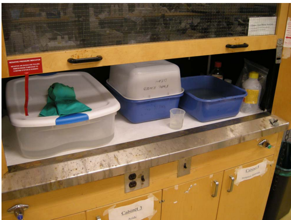
Figure A10.2 – Acid baths used to clean equipment. 10% HCl followed by 5% nitric acid and then DI water
