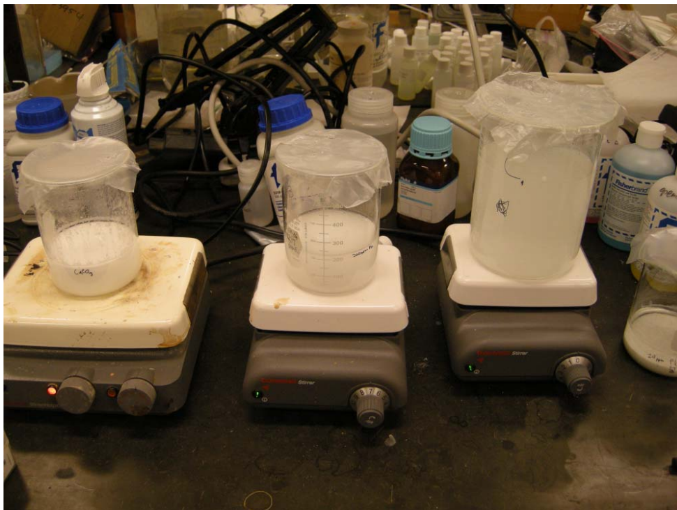
Figure A10.1 – The batch experiments consist of beakers covered with Parafilm and placed on magnetic stirring plates
