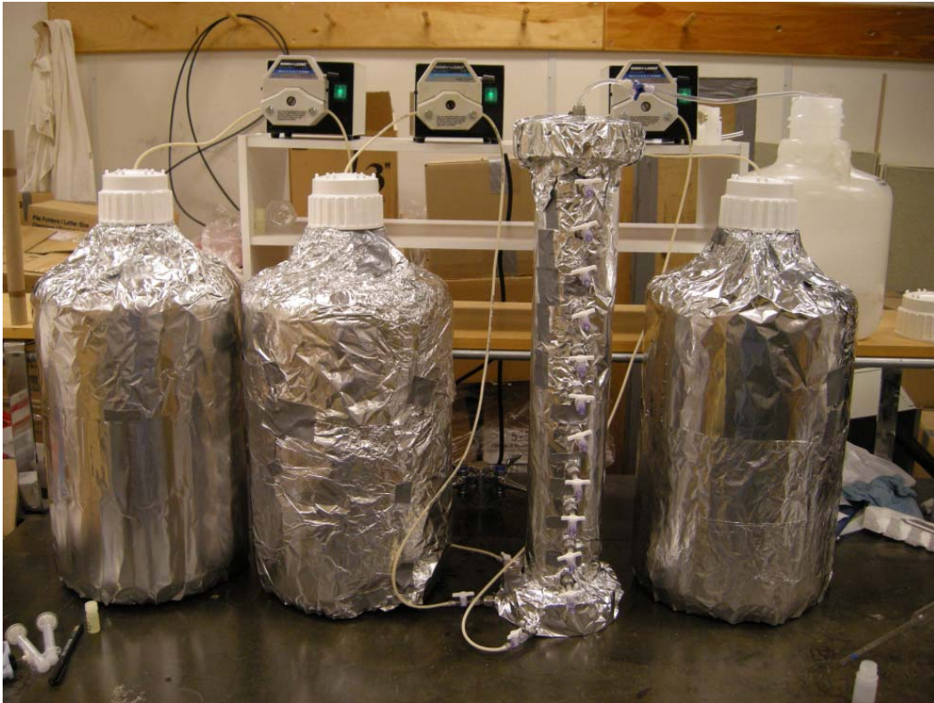
Figure A10.11 – Final setup of the column experiment with everything covered in aluminium foil to prevent bacterial growth
