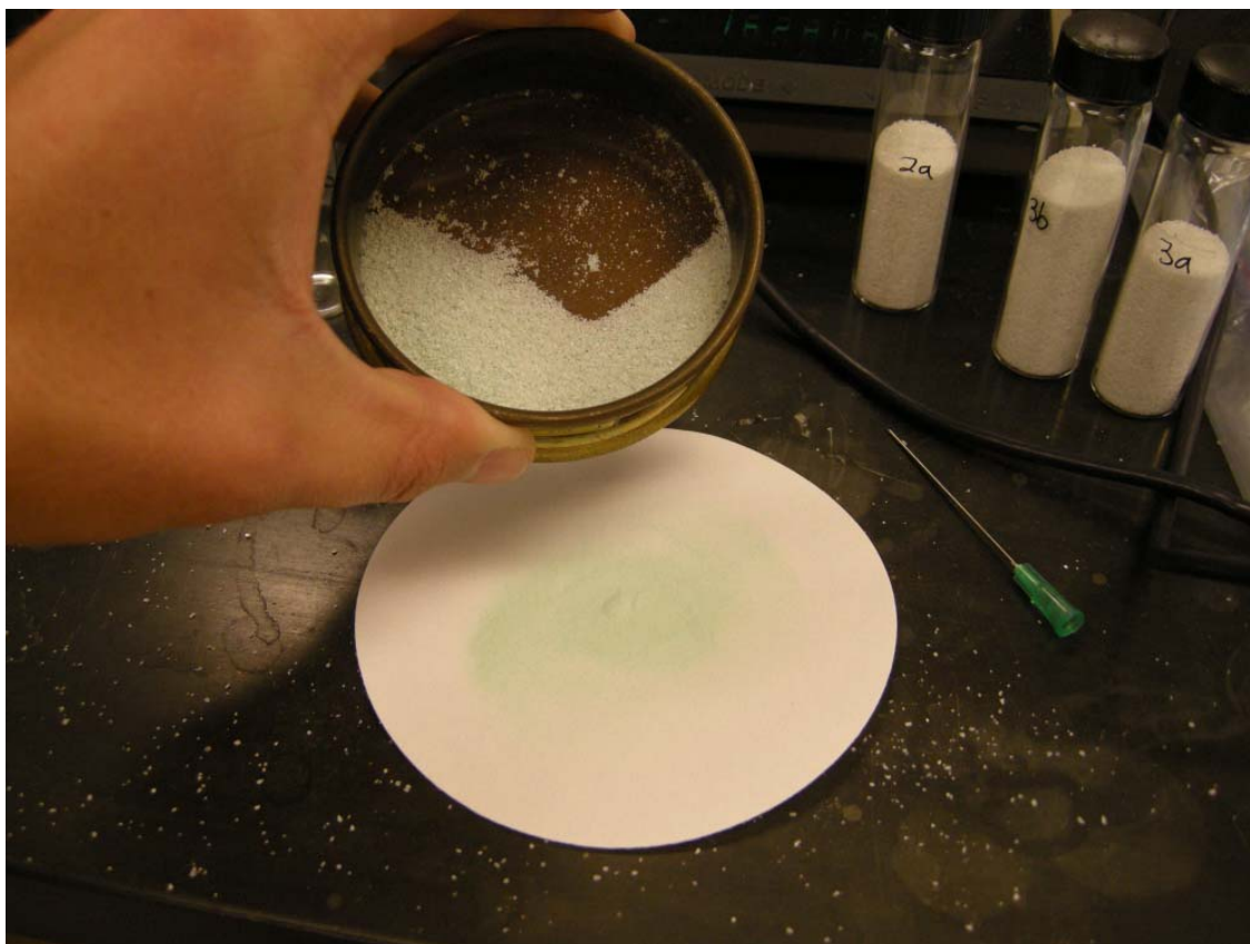
Figure A10.18 – Sieved precipitate for XRD analysis
