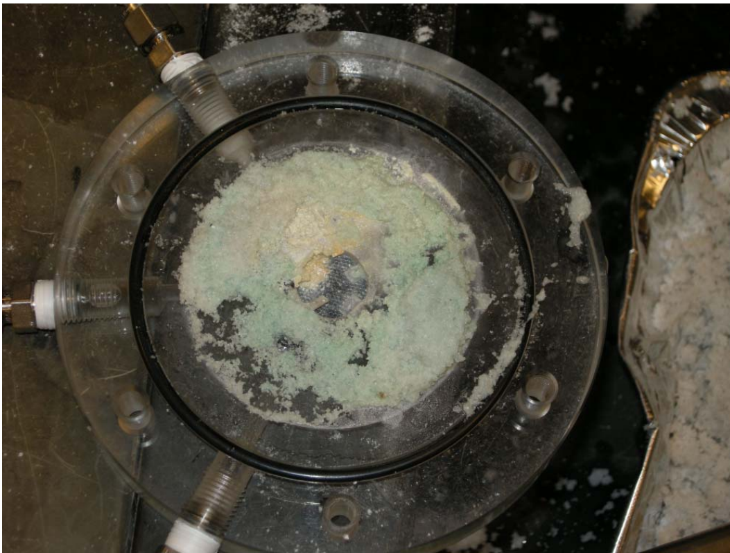
Figure A10.16 – Copper precipitate and yellowish wulfenite directly at the inflow mixing zone
