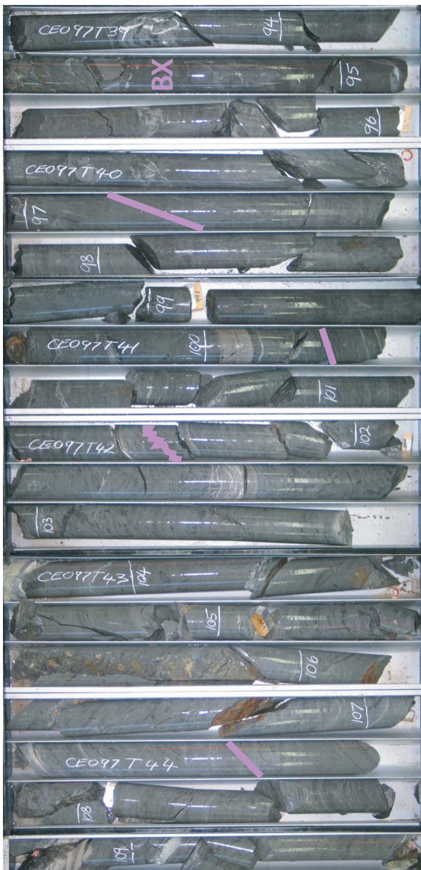
Figure 3.19: Flaser bedded siltstone from drillcore (CE097, 95-109 m). Purple lines indicate bedding orientation. Bedding at 102m is chaotic. At 97m, bedding dips at a steep angle relative to the core axis. At 95m, siltstone-in-siltstone breccia is present. Therefore, it is likely that this drillhole intersects a fault or fold near 96m. This structure is a minor intra-cover feature, rather than a major, basement penetrating fault.
