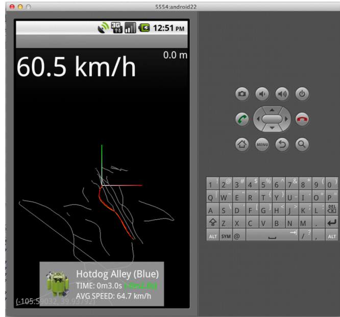
Figure 5.4: This screenshot, taken from the Android emulator depicts the prototype mobile client running on a simulated trajectory. The red track shows the trajectory recorded so far, which is the result of activity recognition detecting a new ski run, while other UI elements tell the user the current GPS parameters. On the bottom, a popup informs the user of the current feature that has been matched using the GIS feature matching operation.
