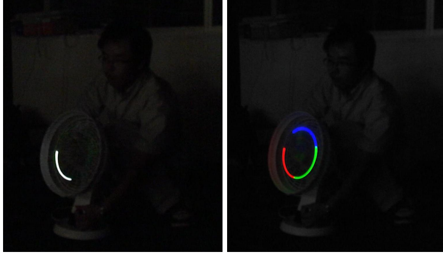
Figure 7.5: Frames from the spinning fan video clip. The left image is a single frame, while the right image shows three consecutive frames in its blue, green and red channel, respectively. The fan’s spinning speed is not constant, but its trajectory is roughly a circle.
