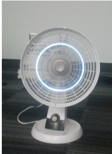
Figure 7.9: The spinning fan photoed by a mobile phone with a 1/8 second exposure. Note that the streak is not a perfect ellipse because the fan has visible jitter.
